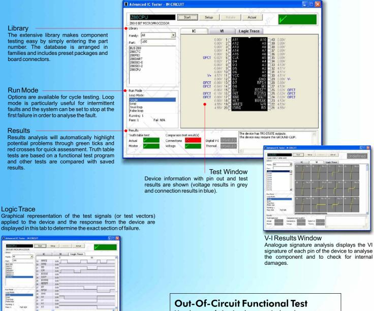
Use the out-of-circuit adapter to isolate the component and to run tests outside the board environment. This is useful to further diagnose a suspect device, to remove the influence of other components or to check a new device before it is placed in-circuit.
