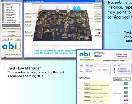
Traceability of information is key to highlighting trends. For instance, repetitive failures of PCB assemblies through a TestFlow may point to a manufacturing defect whilst a board that keeps coming back for repair for the same fault might highlight a design
