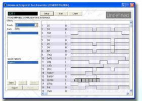
The graphical test generator is the easiest way to create test patterns for individual devices and complete PCB assemblies. Each channel of the ATM can be individually selected to be an input, an output or both (bidirectional). A logic pattern (test vector) can quickly be generated with the use of the mouse.
