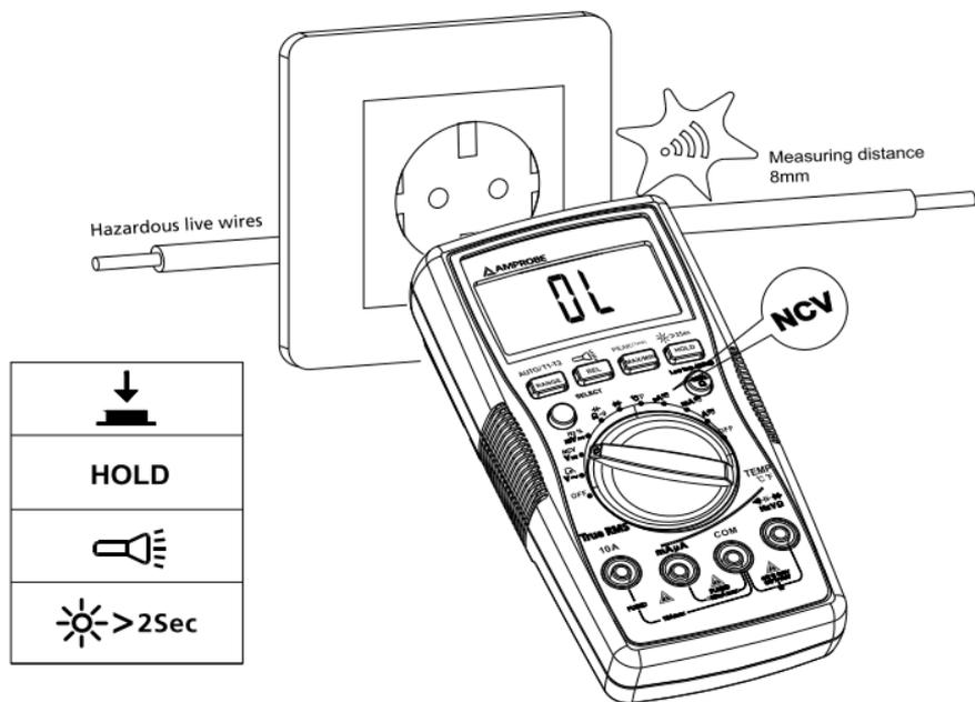
Buzzer will sound when the detected voltage is  $\geq 90V$ , and the buzzer will be on. The distances between the wire and the meter should be  $\leq 8mm$ .
