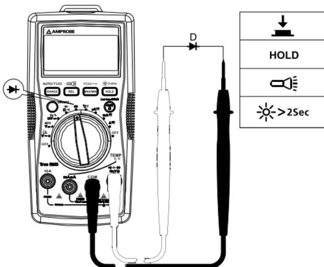
**Note:** A typical junction Voltage drops 0.5 V to 0.8 V.
