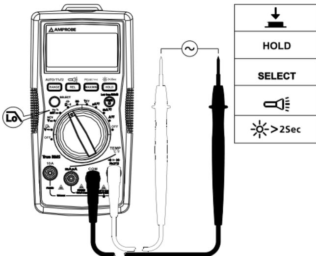
**Note:** The Meter goes into manual mode when Low Pass Filter mode is enabled. Auto-range mode is not available for Low Pass Filter option.
