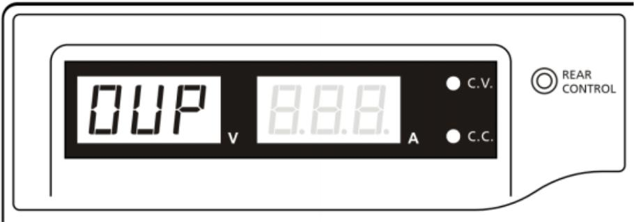
Figure 8 - Overvoltage Protection
