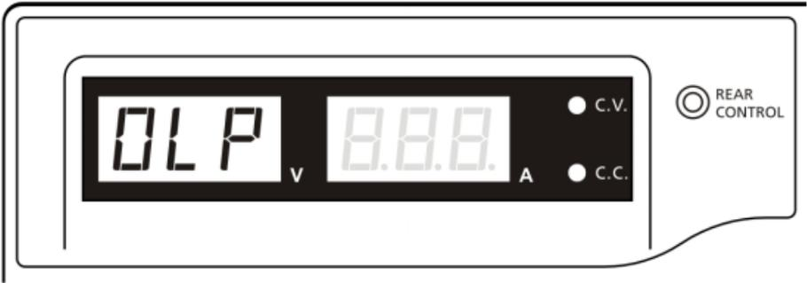
**Figure 10 - Overload Protection**
