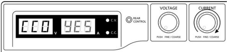
3. Then press the Current Control Knob once to confirm. The "YES" will light up after successfully zeroing current meter offset.
