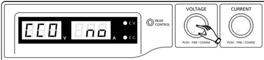
2. Rotate the Current Control Knob until the current meter displays "YES".
