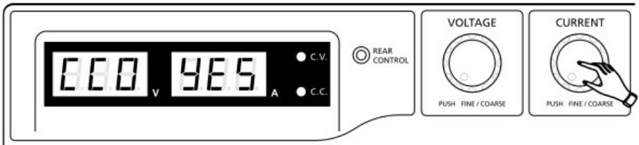
4. Finally, press the Voltage Control Knob to exit.
