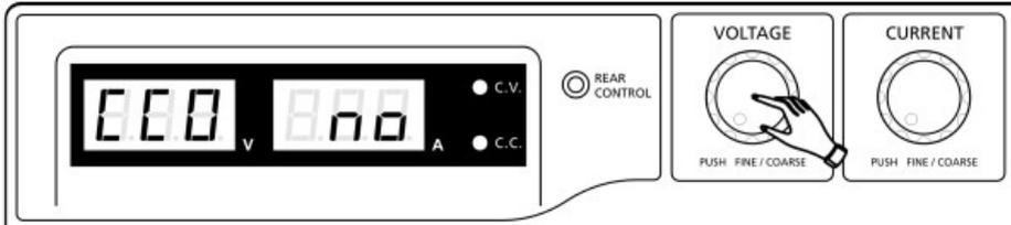
2. When it is showing "CCO", rotate the Voltage Control Knob until voltage meter shows "rPr".
