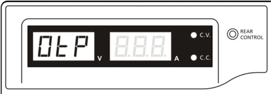
**Figure 9 - Overtemperature Protection**
