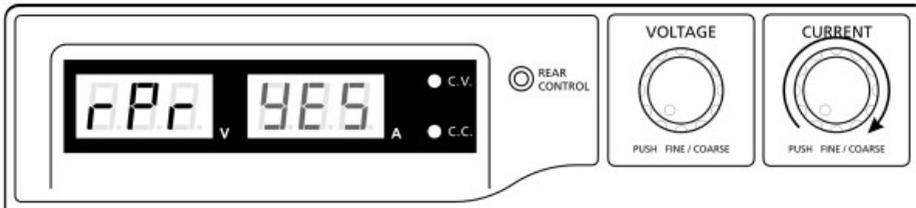
4. Press the Current Control Knob once to confirm. The "YES" will light up after successfully resetting presets to factory default values.
