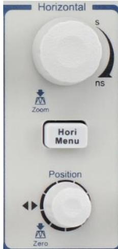
Figure 3.18 – Horizontal Controls
