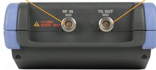
Tracking generators are ideal for tuning filters, determining the usable frequency range of amplifiers and attenuators and aligning receiver IF stages.
