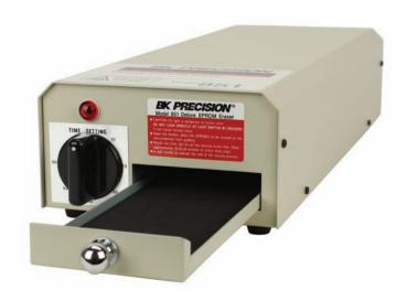
The model 851 is a heavy duty EPROM eraser that can simultaneously erase up to 40 twenty-four pin EPROM's. It is constructed of an all-metal case plus an advanced designed chip drawer that prevents UV radiation from being a hazard to the user. The chip drawer is lined with conductive foam to prevent electrostatic damage to the chips.
