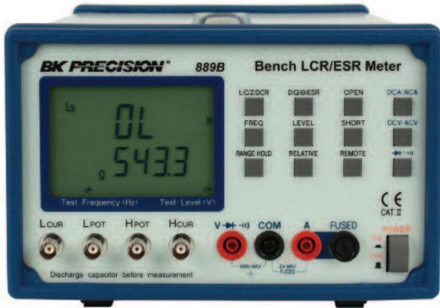
The B&K Precision Corp. 889B Synthesized In-Circuit LCR/ESR Meter is a high accuracy test instrument used for measuring inductors, capacitors and resistors with a basic accuracy of 0.1%. Also, with the built-in functions of DC/AC Voltage/Current measurements and Diode/Audible Continuity checks, the 889B can not only help engineers and students to understand the characteristics of electronics components but also being an essential tool on any service bench.
