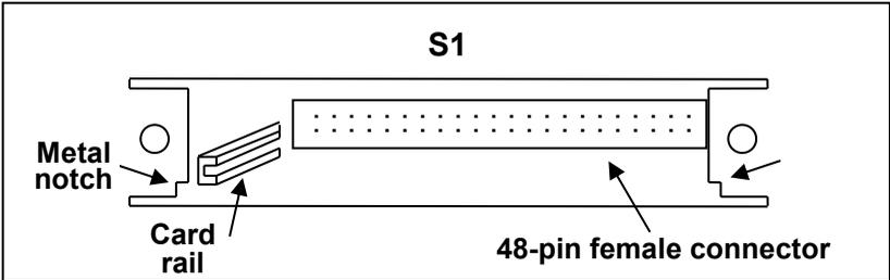
3. The interface card should go right below the metal notches on both sides and fit in between the inner card rails, also on both sides. Slide the card down carefully. When it touches the 48-pin connector, slowly push the card all the way in until the panel of the interface card aligns with the rear panel of the power supply.
