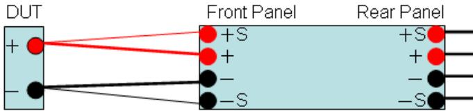
**Figure 17- Front Panel Remote Sense Setup**
