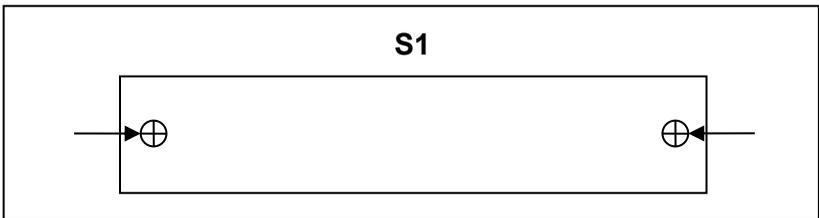
2. Use a flat blade screwdriver to gently pry the left and right side of the interface card plate. When there is enough room, use the screwdriver to pry the top part of the card until the card has slid out with enough room to pull out the card by hand.
