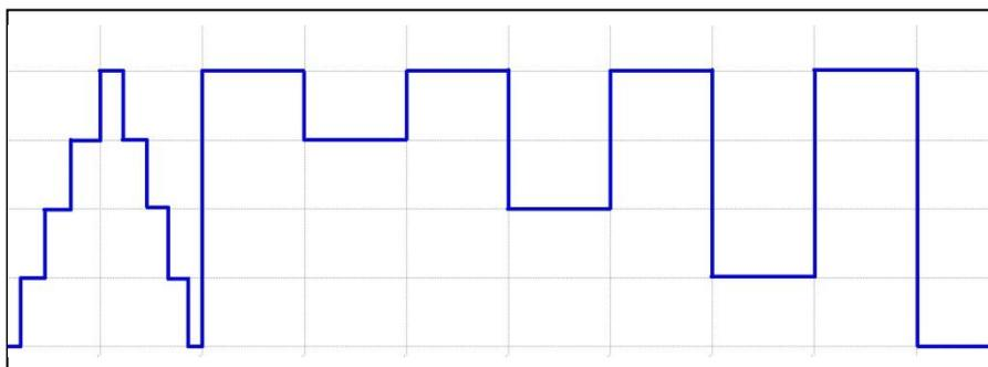
To execute example 2 sequence after example 1 sequence, then modify sequence of example 1 with NEXT 2 command. Send the following steps to modify and execute the program to generate a waveform sequence shown above.
