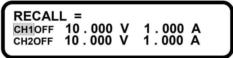
2. Use the keypad to enter the memory location that contains the voltage and current values to recall. The voltage and current settings will change immediately to the recalled settings.
