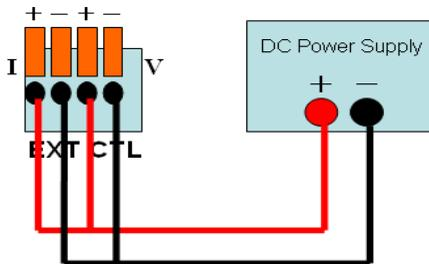
Figure 36- Single Channel Analog Control Calibration Setup
