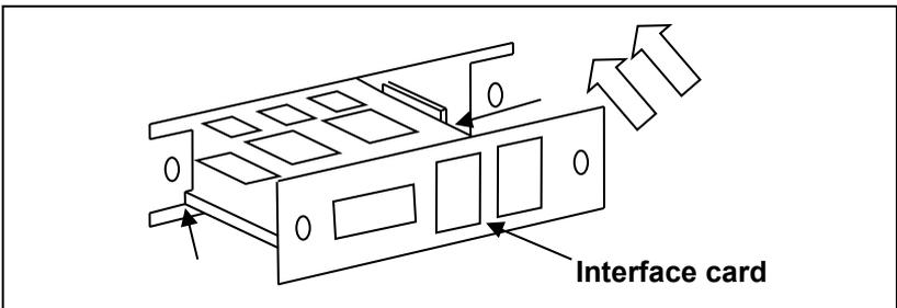
4. Place the two screws to tighten and secure the installed card.
