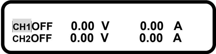
5. Press **OUTPUT** to turn the output ON (enabled), and output voltage and current will change as your external DC voltage sources or resistances change.
