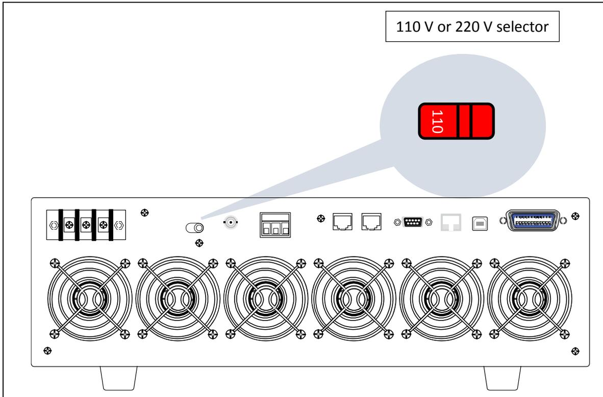
Figure 12 - Line Voltage Selector Location 9803/9805
