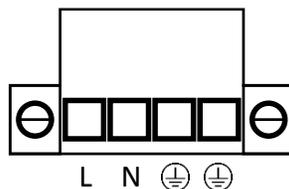
Figure 20 – Rear Panel AC Output Terminal
