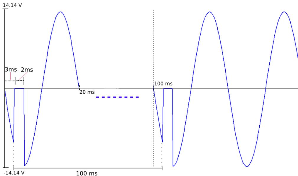
Figure 26 – Dropout Waveform
