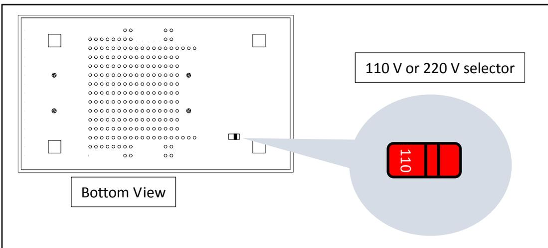
Figure 11 – Line Voltage Selector Location 9801
