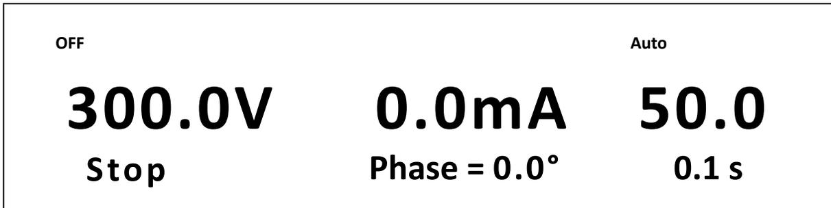
Use the numeric keys to set the stop phase angle and press
