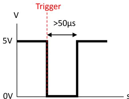
Figure 22 - TTL Pulse Width
