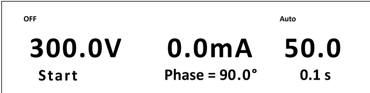
Use the numeric keys to set the start phase angle and press
