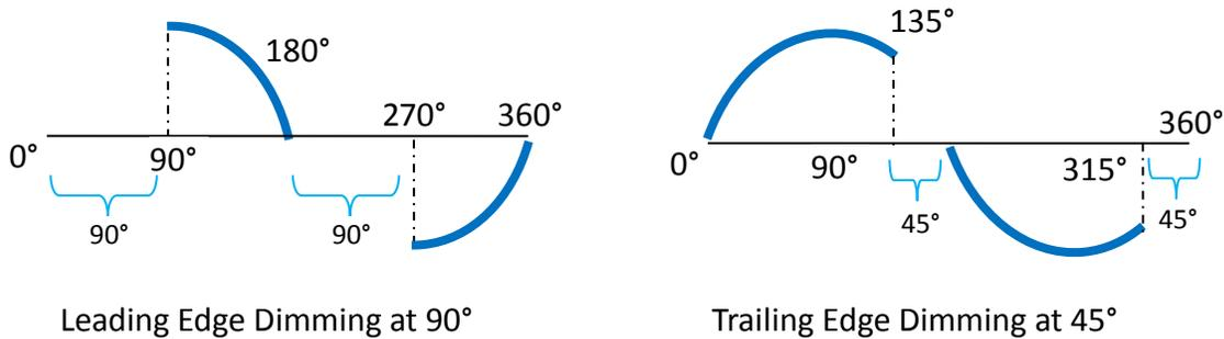
Figure 24 – Leading and Trailing Edge Dimming
