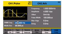
These instruments are capable of many different types of modulation for various applications. Modulate your waveforms with AM, DSB-AM, FM, PM, ASK, FSK, and PWM modulation schemes.
