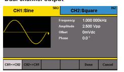
Save time with the 4060 Series' two independent channels to output synchronous signals. With a push of a button, all waveform parameters can be quickly copied between channels to set up identical output signals. Phase between channels can also be adjusted from the front panel.
