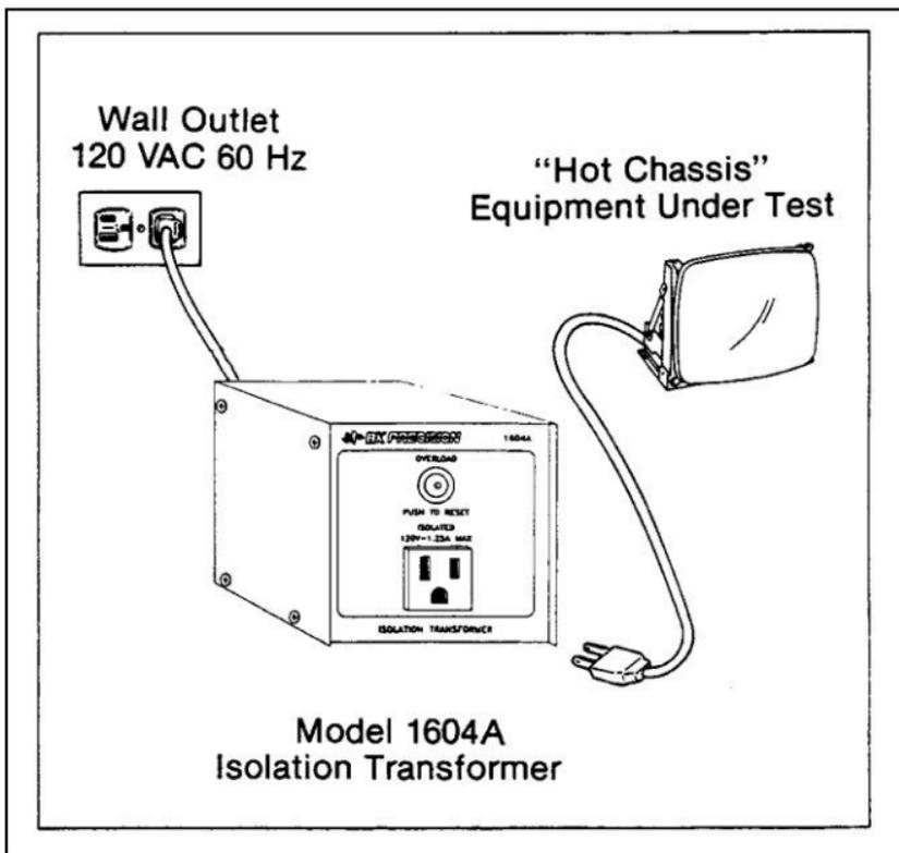
1. Connect power plug of Model 1604A Isolation Transformer to 120 volt, 60 Hz ac wall outlet
