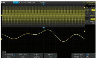
Capture longer time periods at higher resolution with a maximum memory depth of 14 Mpts. Enable zoom feature to display specific events in more detail.
