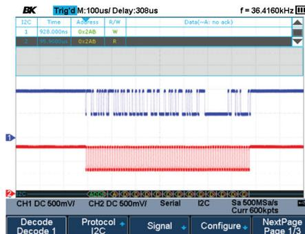
Decoding mode displays the serial bus data through the events list. Bus protocol information can be quickly and intuitively displayed in a tabular format.
