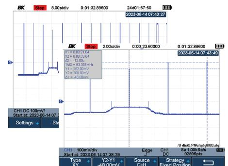
Use sample logging to monitor and analyze long-term signal behavior by recording data continuously at up to 25 kSa/s. This mode allows recorded data to be played back for post acquisition analysis.
