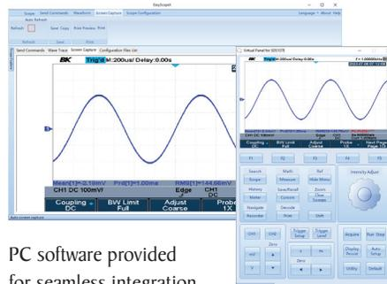
PC software provided for seamless integration between the oscilloscope and PC. Capture and transfer waveforms, screen images, setups and measurement results to a PC via the USB device port.
