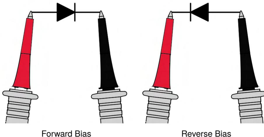
**Figure 2.6** Testing Diodes
