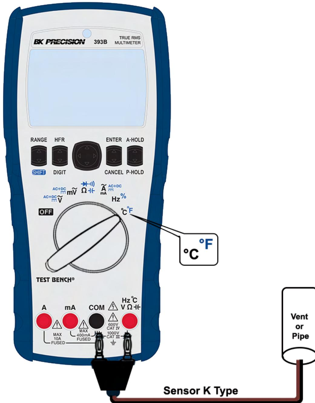
Figure 2.10 Temperature Measurement
