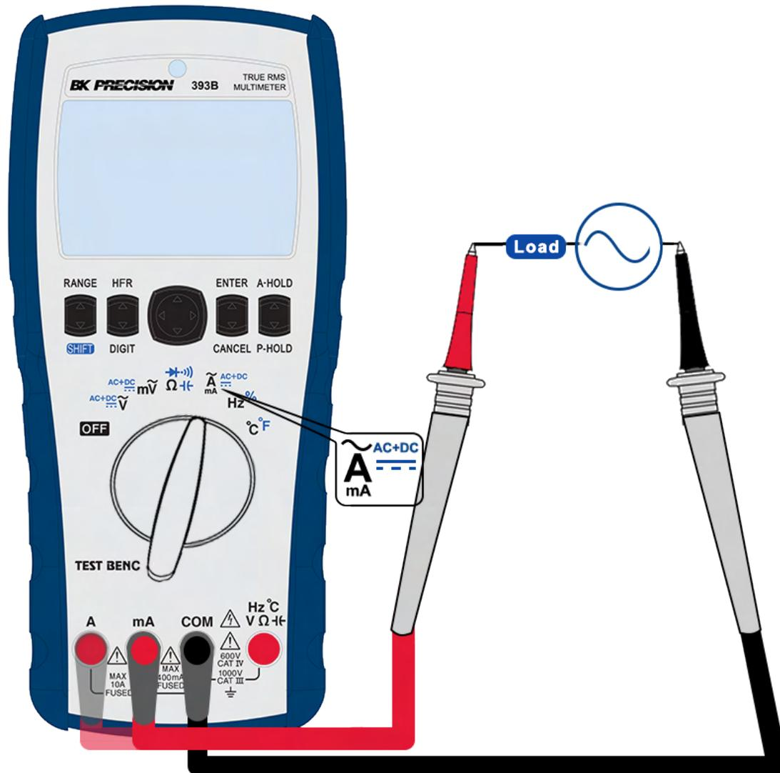
Figure 2.8 Current Measurement
