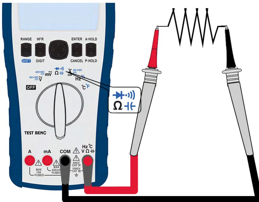
**Figure 2.5** Resistance Measurement
