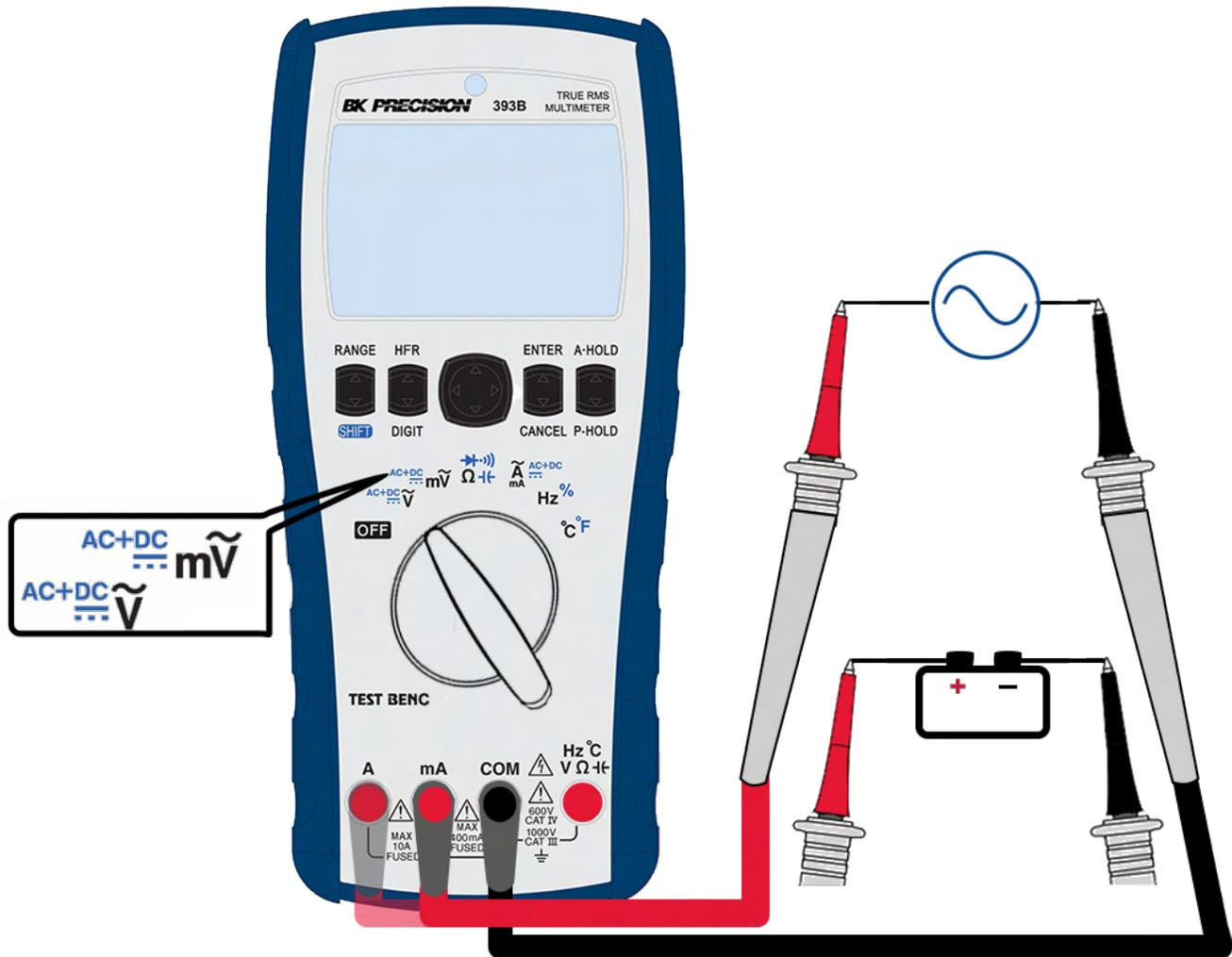
**Figure 2.1** Voltage Measurement
