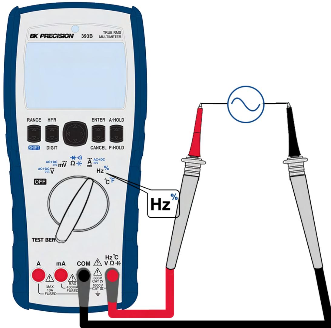
Figure 2.9 Frequency Measurement
