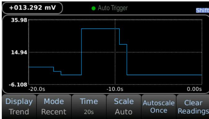
The trend chart plots data as a trend line over time. The mode can be changed to display recent data where the time in seconds before present can be adjusted. Press the 'Scale' softkey to then select 'Manual' and use the directional keypad to adjust top/bottom boundaries.
