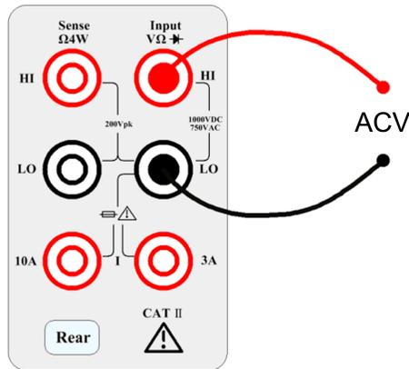
**Step 2:** Press the ACV button on the front panel to enter the ACV function interface.
