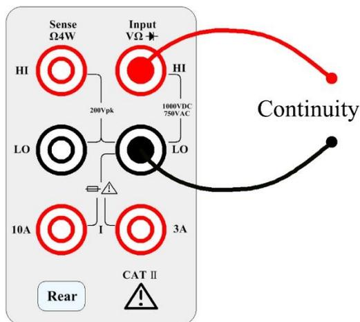
**Step 2:** Press **Cont** on the front panel to open a menu that specifies whether the digital multimeter will beep to indicate the continuity.
