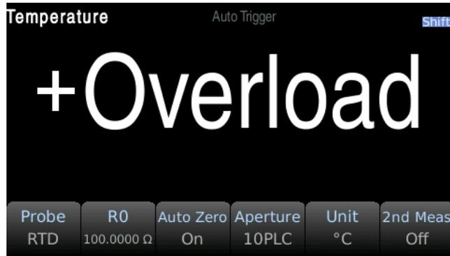
**Step 3:** Press Probe to select the probe type. If you choose to use RTD, this menu will have a softkey to specify the resistance of the RTD at 0 degrees Celsius (R0).
