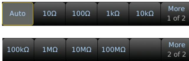
Press Range and select the range. Auto range (Auto) can automatically select the appropriate range for measurement based on the input signal. The auto range is adjusted upwards to 110% of the existing range and down to 10% of the existing range.
