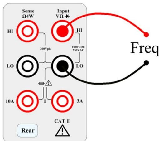
**Step 2:** Press the
