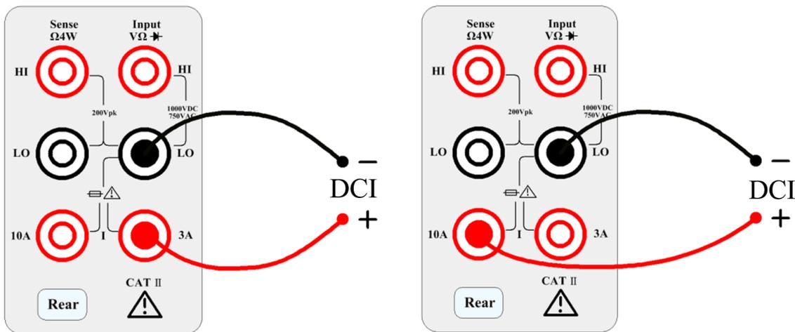
Use the 10 A terminal for current measurements greater than 3 A.
