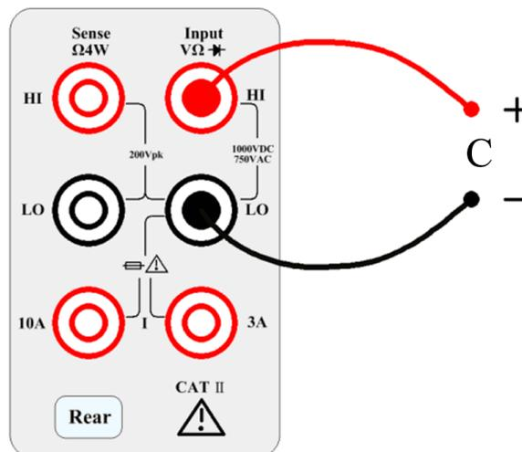
**Step 2:** Press
