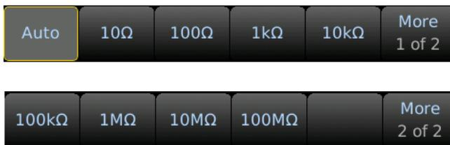
Press Range and select the range. Auto range (Auto) can automatically select the appropriate range for measurement based on the input signal. The auto range is adjusted upwards to 110% of the existing range and down to 10% of the existing range.
