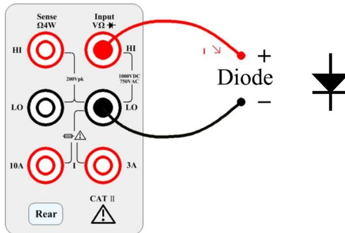
**Step 2:** Press **Shift** then press **Cont** on the front panel to enter the diode test interface.
