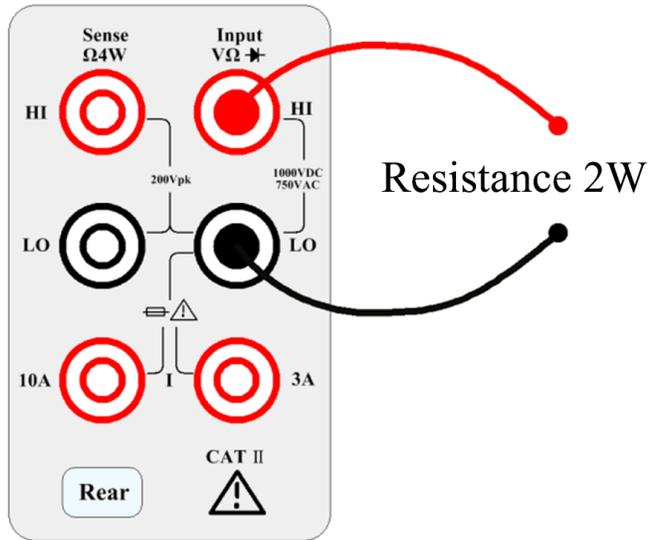
**Step 2:** Press  $\Omega 2W$  on the front panel to enter the two-wire resistance test interface.
