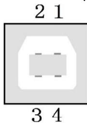
This unit uses a USB-B type interface, which can communicate via a standard square USB interface cable. There are no settings in the menu system for USB configuration. The only requirement is that a USBTMC driver is installed. A USBTMC driver is included with VISA software.
