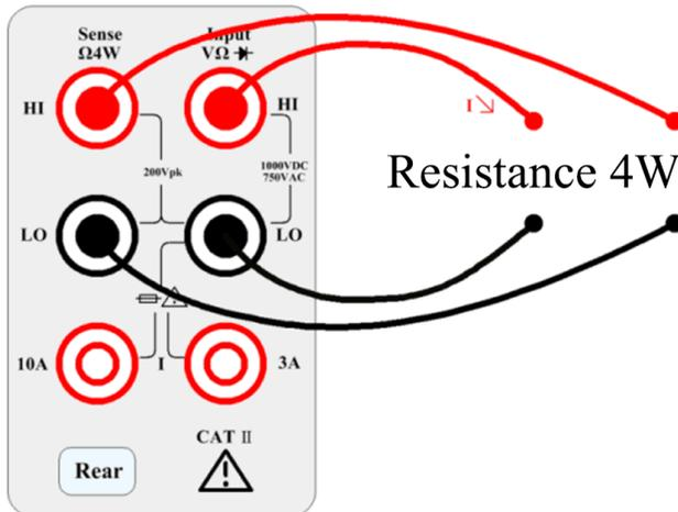
**Step 2:** Press **Shift** then press **Ω2W** on the front panel to enter the four-wire resistance test interface.
