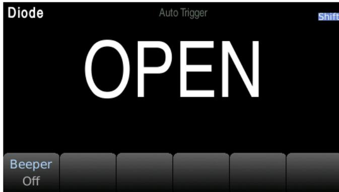
When converted to a 0.3V to 0.8V threshold, the instrument beeps (if a beep is enabled). A voltage of 0 to 5V is displayed on the front panel. When the measured break-over voltage is greater than 5V, the front panel will display OPEN.
