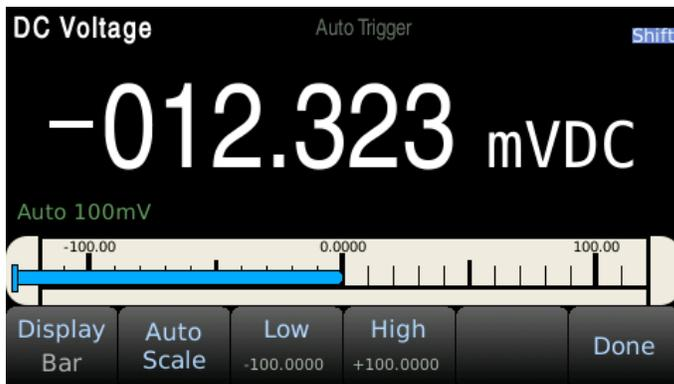
The bar meter displays live measurements on a horizontal bar graph. Press 'Auto Scale' to automatically adjust the upper and lower limits or set the limits manually using. Use the softkeys and directional keypad to adjust the Low/High values.
