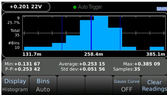
The histogram display mode groups data into bins represented graphically in vertical bars. By default the Bin count is set to Auto. The Bin count can be changed manually to 10, 20, 40, 100, 200, or 400. When using manual Bins, the high/low bounds can be adjusted using the directional keypad. When statistics are displayed in histogram mode, the dark blue line in the middle represents the average, and the outside blue lines represent one standard deviation from the average.
