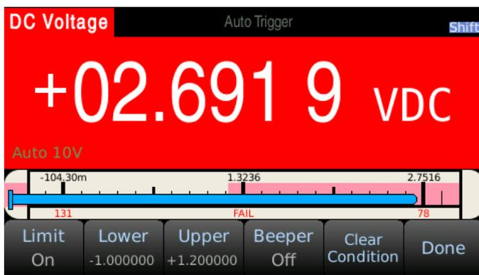
The bar meter display mode can also be enabled with Limit mode. The upper and lower limits are displayed on the bar meter in red.
