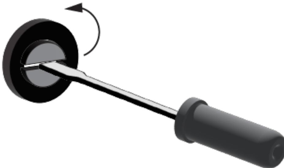
**Figure 2.1** Fuse Removal
