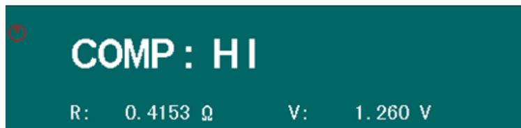
Figure 3.18: Compare Test - Above Limits
