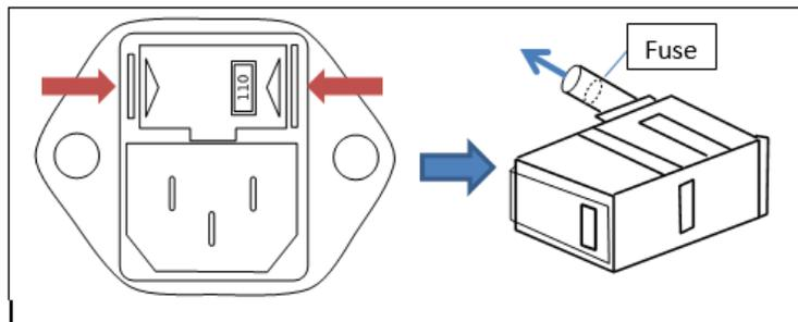
Figure 2.1: Change Line Voltage Configuration
