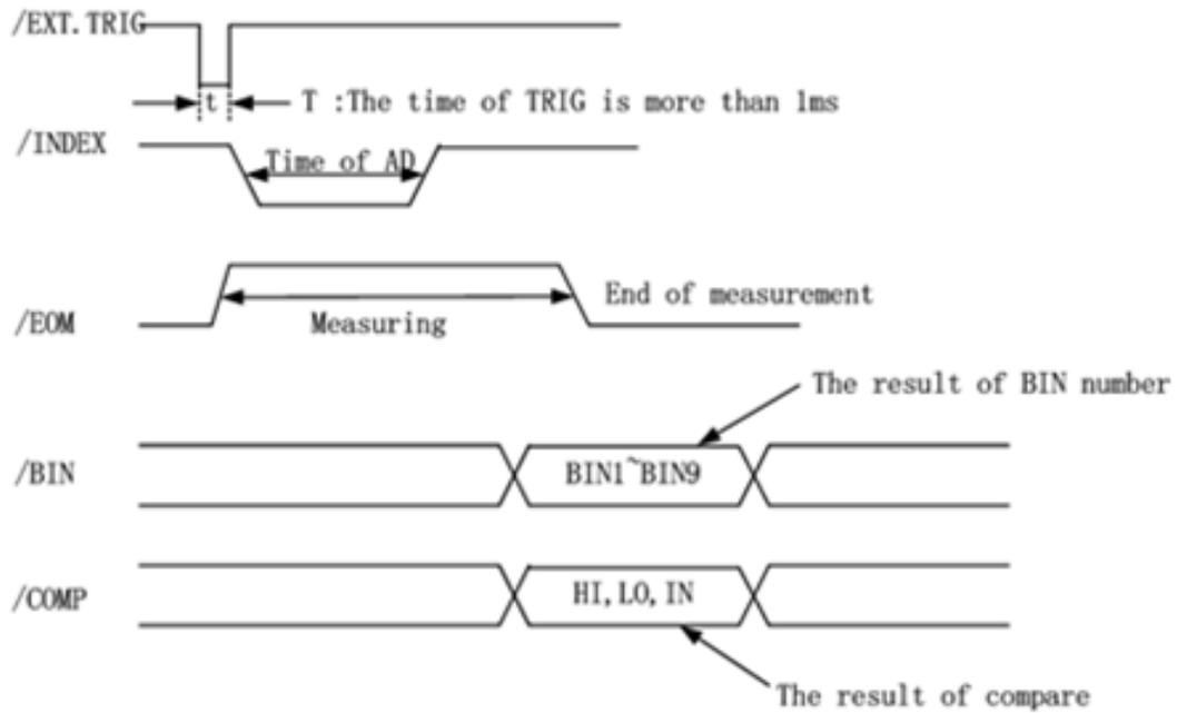
Figure 5.2: Handler Interface Timing
