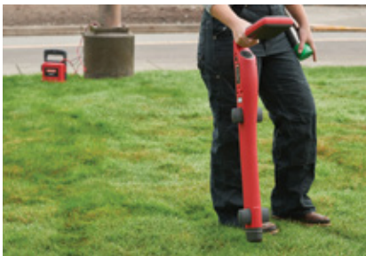
Trace an individual utility by connecting the transmitter directly with the test leads
