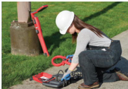
The Transmitter will automatically change modes based on which accessory is plugged in
