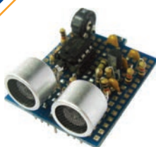
ARX-ULT ARX Ultrasound Distance Measurement
