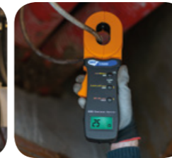
Earth resistance measurement with clamp T2100.
