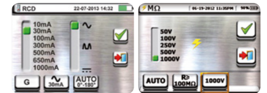
Selection of RCD type and tripping current.
