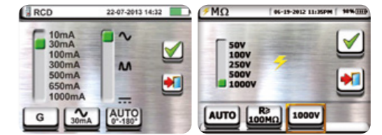
Selection of RCD type and tripping current.
