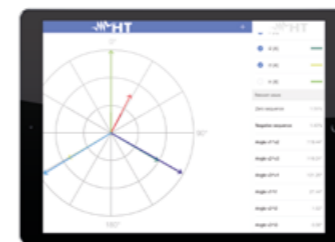
Example of display Real-time phasors
