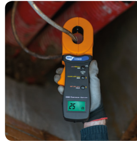
Measurement of earth resistance with Clamp T2100.
