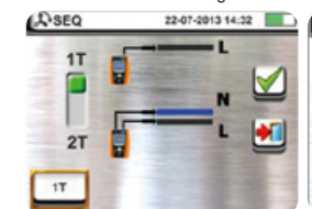
Selection of measurement type of phase sequence.
