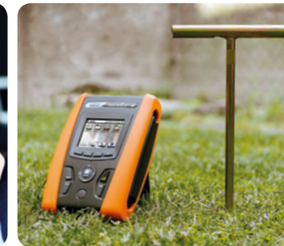
Measurement of earth impedance by voltammetric method.
