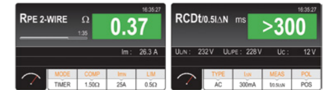
2-wire continuity test
