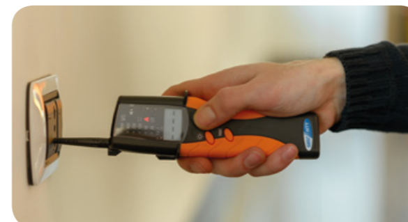
Phase detection function through conductive button.
