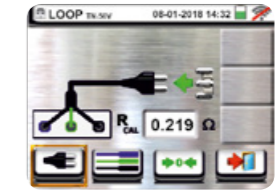
ZeroLoop: compensation of the resistance of the test cables used for Loop impedance measurement.
