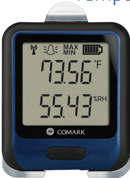
The Diligence™ WiFi RF313-TH data logger measures and records temperature and humidity via internal sensors.
