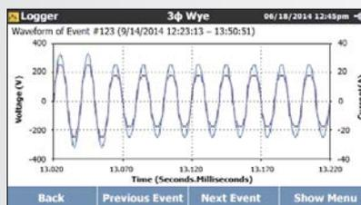
Capture voltage events and inrush currents with pre-defined thresholds
