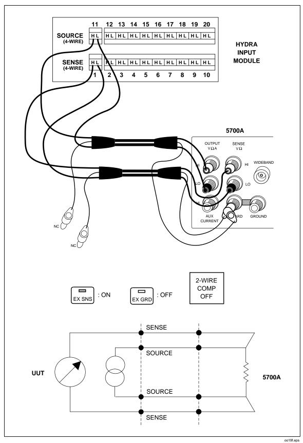
Figure 6-2. 4-Terminal Connections to 5700A
