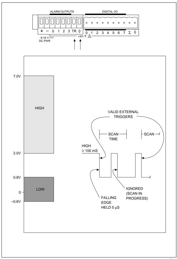
Figure 5-1. External Trigger Timing
