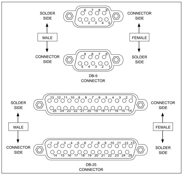
Figure F-6. RS-232 DB9 and DB-25 Connectors
