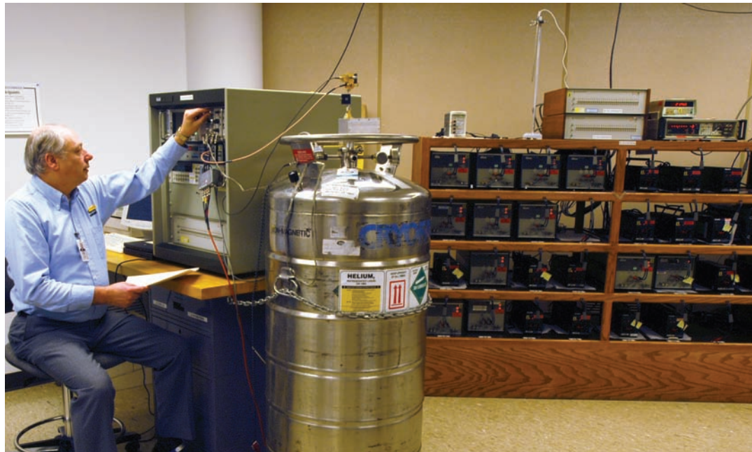
The Fluke Josephson Voltage System in Everett, Washington USA. Fluke laboratories in the United States and Germany house 2 of only 35 Josephson dc voltage arrays in the world found outside a national laboratory.
