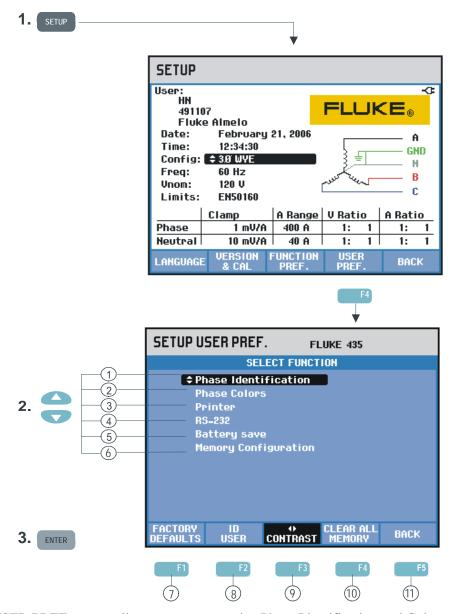
USER PREFerences allows you to customize Phase Identification and Colors, Printer and RS-232 settings, Auto shut-off, Memory Configuration, definition of User name/address (as shown in entry screen), and display contrast. Many menus have a function key to reset to factory default settings.
