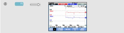
All readings are recorded during logging, but not all of them are visible at a time. Press Function key F1 to assign the up/down arrow keys to select another set readings.
