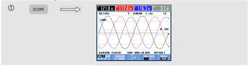
The Scope Waveform screen offers an oscilloscope style of display of voltage and/or current waveforms with a fast update rate. The screen header shows the related rms voltage/current values (10/12 cycle rms or 150/180 cycle rms as per IEC61000-4-30:2003). As a default 2 waveform periods are displayed. Channel A (L1) is the reference channel and 2 complete cycles starting at 0 volt are displayed.
