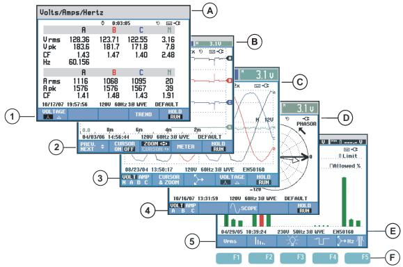
Figure 5-1. Survey of Display Types
