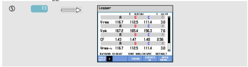
This screen displays all current readings of the logger function. Use up/down arrow keys to scroll across the Meter screen.
