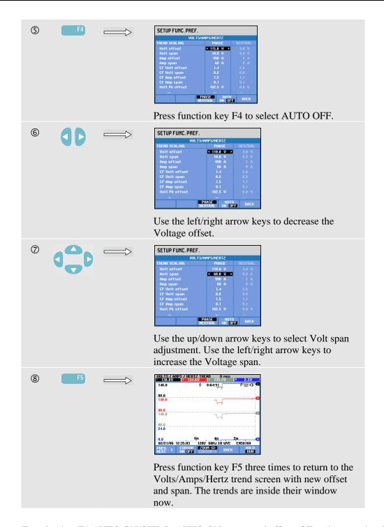
Function key F4 AUTO ON/OFF. In AUTO ON, range and offset of Trends are updated automatically on every new acquisition to make them fit closely within the available window. Manual adjustment is possible if Function Key F4 is set to AUTO OFF
