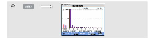
The Bar Graph display shows the percentage contribution of each of the components related to the full signal. A signal without distortion should show a 1<sup>st</sup> harmonic (= the fundamental) at 100 % while the others are at zero: in practice this will not occur because there always is a certain amount of distortion resulting in higher harmonics.
