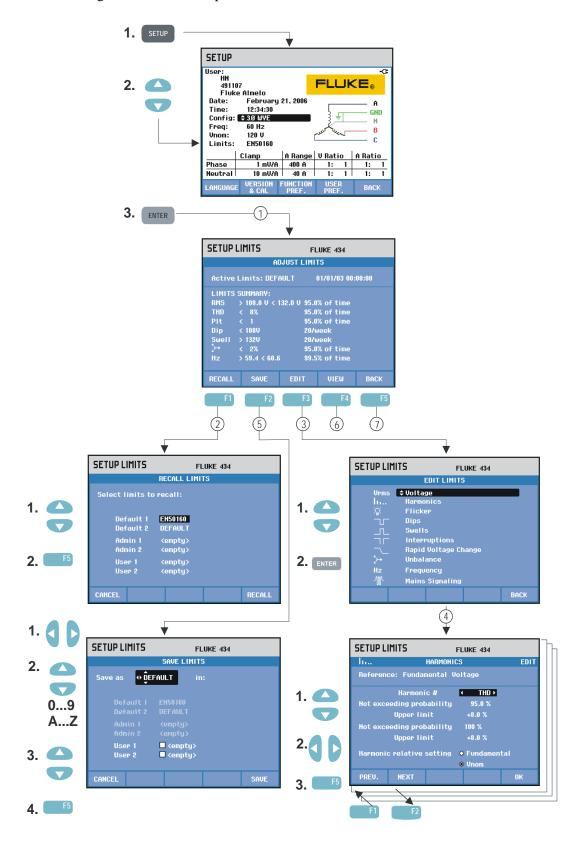
Limits Adjustments is used to save, recall, and define sets of limits for:
