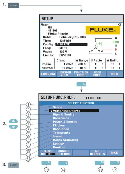
FUNCTION PREFerences allows you to customize data presentation of measuring functions. This concerns for instance Offset and Span of Trend and Waveform displays. The entry menu is available in the selected information language. The table below gives a survey adjustable items for each function. A measuring function stays active while you adjust its settings. This allows you to directly judge the result of the adjustment.
