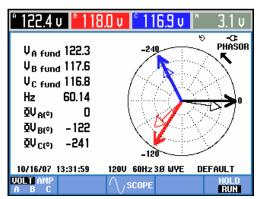
Figure 6-3. Vector diagram for correctly connected Analyzer
