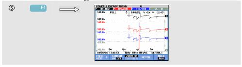
The figures in the Meter screen are instantaneous values that update constantly. Changes in these values over time are recorded whenever the measurement is active. All values in the Meter screen are recorded, but the Trends from each row in the Meter screen are displayed one at a time. Press function key F1 to assign the arrow keys to row selection.
