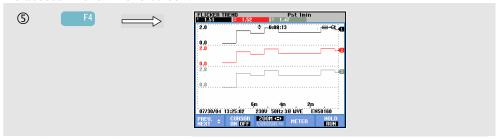
The parameters in the Meter screen update over time. They are recorded whenever the measurement is on. Trend displays the changes in these values over time. All values in the Meter screen are recorded, but the Trends from each row in the Meter screen are displayed one at a time. Press function key F1 to assign the arrow keys to row selection. The Trend display may consist of 6 screens.
