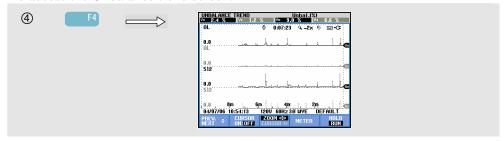
The figures in the Meter screen are instantaneous values that update constantly. Changes in these values over time are recorded whenever the measurement is active. All values in the Meter screen are recorded, but the Trends from each row in the Meter screen are displayed one at a time. Press function key F1 to assign the arrow keys to row selection. The Trend display may consist of 6 screens.
