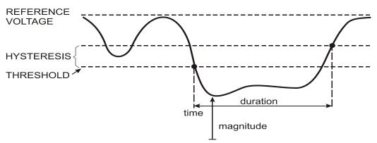
Figure 9-1. Characteristics of a voltage dip
