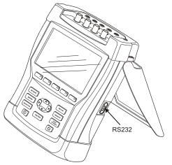
Figure 4-1. Tilt stand and location of RS-232 interface
