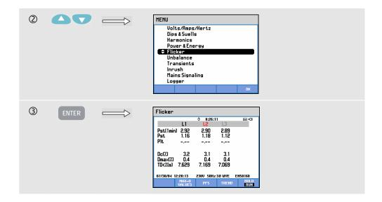
Flicker is characterized by: short term severity Pst (measured over 1 min for fast feedback), short term severity Pst (measured over 10 min) and a long term severity Plt (measured over 2 hours). This data and also the related D-parameters Dc, Dmax, and TD (acc. to EN61000-3-3) are displayed in the Meter screen.
