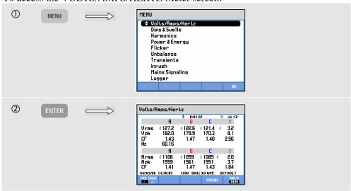
The Meter screen gives an overview of voltages and currents in all phases. Also frequency and Crest Factors are shown. The Crest Factor CF indicates the amount of distortion: a CF of 1.41 means no distortion and higher than 1.8 means high distortion. Use this screen to get a first impression of power system performance before examining the system in detail with other measuring modes. The number of columns in the Meter screen depends on the power system configuration.
