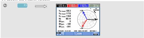
The Phasor screen displays the phase relation between voltages and currents in a vector diagram. The vector of reference channel A (L1) points in the positive horizontal direction. Additional numerical values are fundamental phase voltage, frequency, and phase angles. The screen header shows rms voltage and/or current values.
