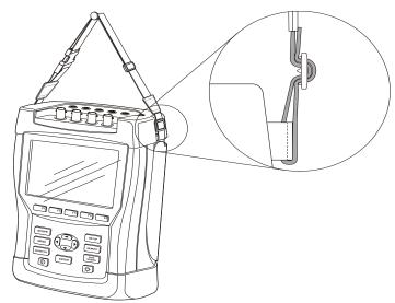
Figure 4-2. Fixing the hang strap
