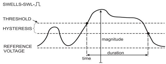
Figure 9-2. Characteristics of a voltage swell
