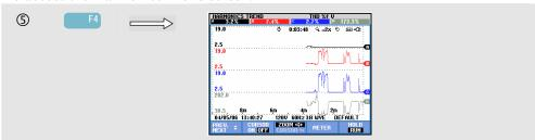
Trend shows how harmonics vary over time: Cursor and Zoom can be used to investigate details. All values in the Meter screen are recorded, but the Trends from each row in the Meter screen are displayed one at a time. Press function key F1 to assign the arrow keys to row selection.
