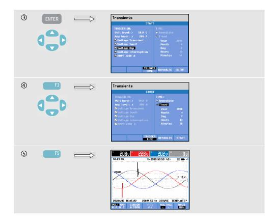
In the Start menu you can choose a trigger event or a combination of trigger events, transients (Volt) and current (AMP) trigger level, and Immediate or Timed start of the measurement.
