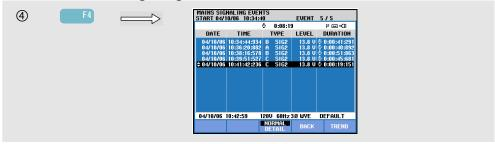
The events table shows in Normal mode the events (V3s above the limit) that occurred during the measurement. Date, time, type (phase, signal 1 or signal 2), level and duration of each event are listed. In Detail mode additional information is given on threshold crossings.
