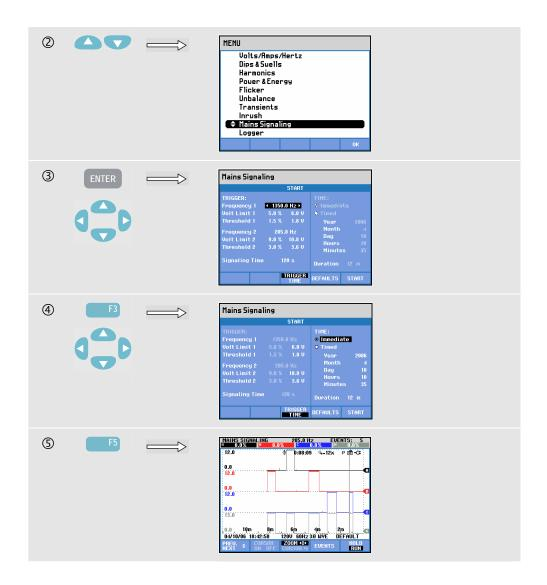
The traces build up from the right side. Readings in the header correspond to the most recent values plotted on the right. With the up/down arrow keys you can select readout as a percentage of nominal line voltage or as a 3 second average voltage (V3s). The Neutral conductor is not used for Mains Signaling, but is shown for troubleshoot purposes.
