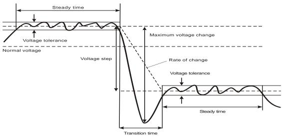
Figure 9-4. Characteristics of a rapid voltage change
