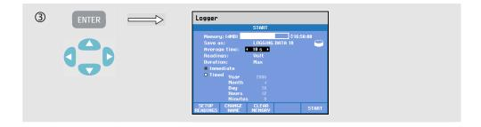
The set of readings to be logged is selectable in the menu under function key F1-SETUP READINGS. With the up/down arrow keys you can select five sets of predefined readings (Default 1-5) and two sets of user definable readings (User 1, 2). Table 17-1 gives an overview of the readings available under Default  $1 \dots 5$ . This also gives you an impression of the readings available for logging.
