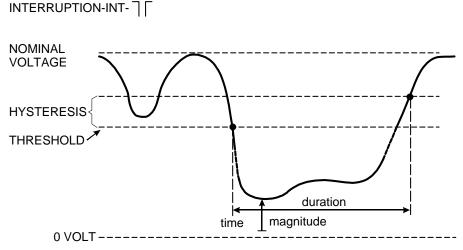
Figure 9-3. Characteristics of a voltage interruption
