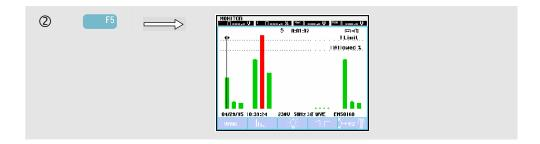
Power Quality Monitoring is reached via the MONITOR key and a menu for Immediate or Timed start. With the left/right arrow keys you can position the Cursor on a particular Bar Graph. Measuring data belonging to the bar is shown in the screen header.
