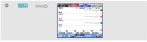
All values in the Meter screen are recorded, but the Trends from each row in the Meter screen are displayed one at a time. Press Function key F1 to assign the up/down arrow keys to row selection.
