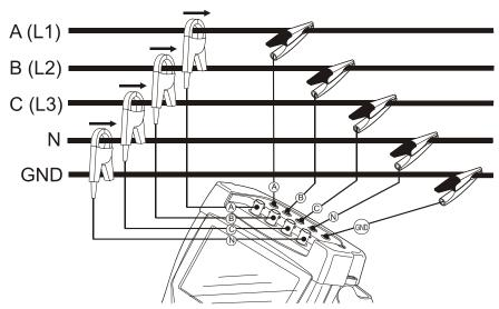
Figure 6-2. Connection of Analyzer to 3-phase distribution system
