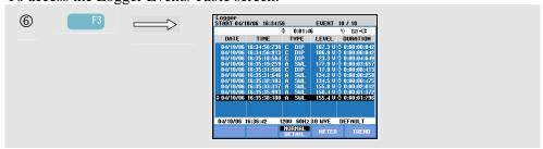
The Events table lists all threshold crossings of phase voltages. Thresholds according to international standards or user-definable thresholds can be used. Threshold adjustment is reached via the SETUP key and Limits. For detailed information see Chapter 20, Limits Adjustments.
