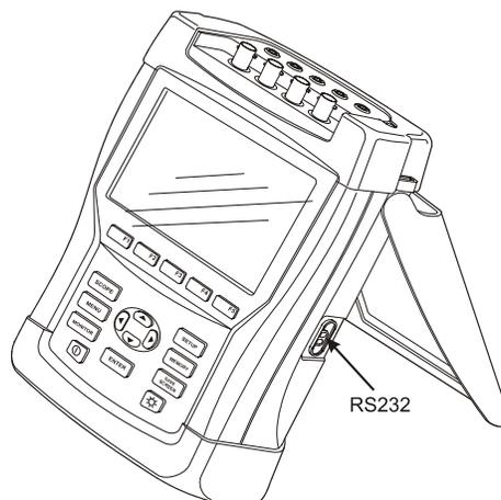
**Figure 4-1. Tilt stand and location of RS-232 interface**
