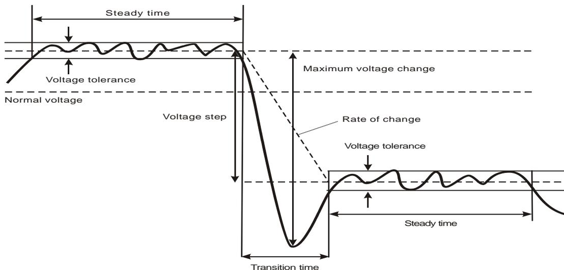
Figure 9-4. Characteristics of a rapid voltage change
