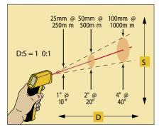
The single dot laser system indicates the approximate center of the measurement area.
