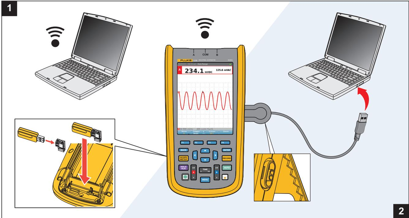
Figure 2. 120B ScopeMeter Test Tool to PC Communication
