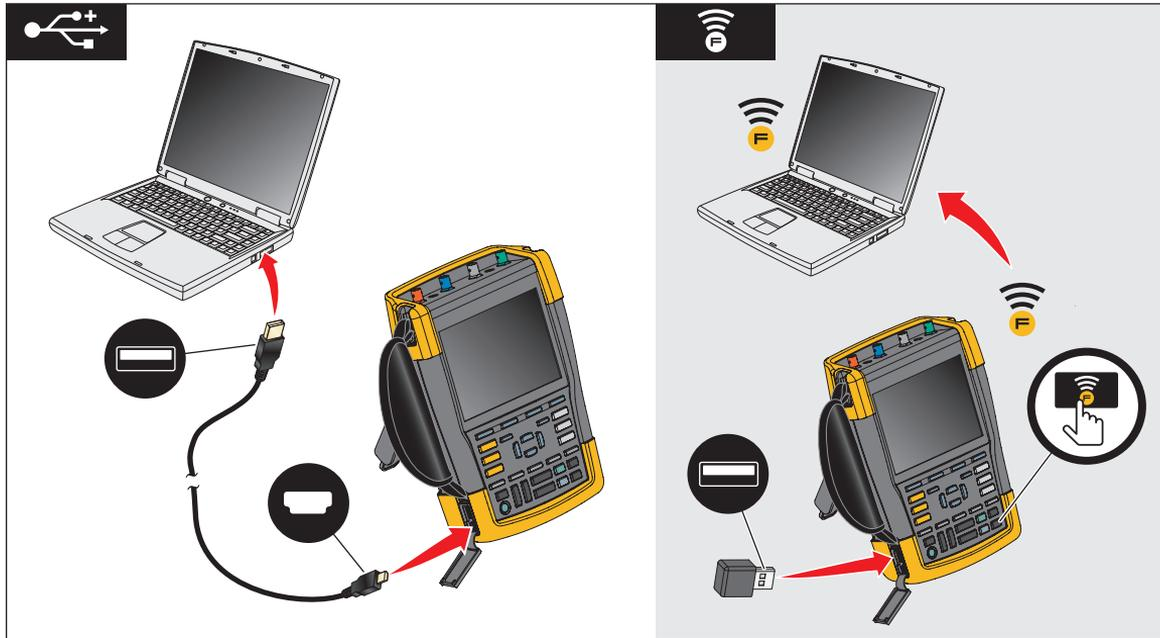
Figure 1. Test Tool to PC Connections
