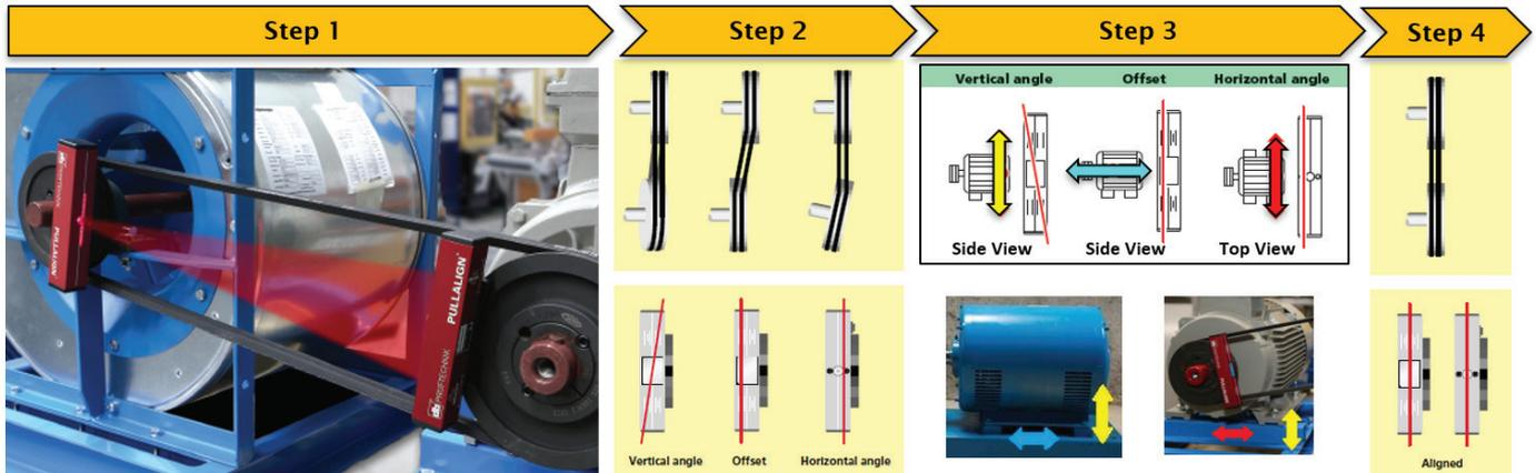
1. Initiate the PULLALIGN® laser and mount the units on the faces to be aligned.
