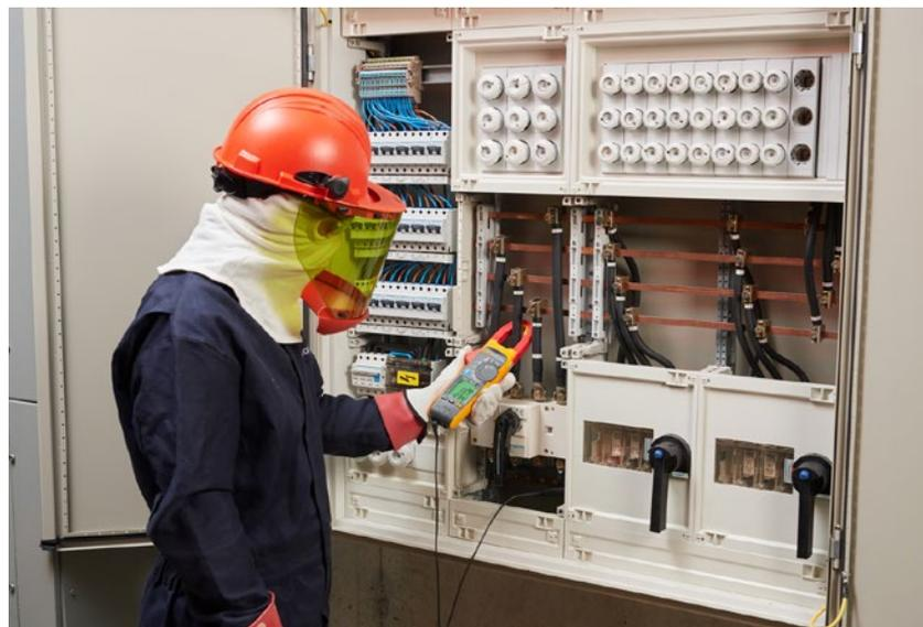
Fluke 378 FC Clamp Meter taking measurements in a panel.
