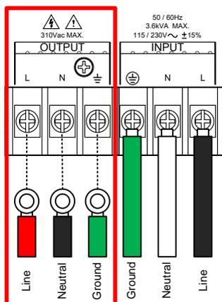
APS-7100E shown. The input terminals are already connected and shows which output terminals are to be connected.
