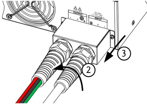
4. Remove the AC power cord wires.
