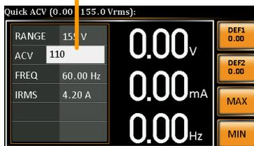
Using the Arrow Keys and Scroll Wheel to edit parameter values
