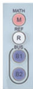
The GDS-3000 Series provides two dedicated keys in the front panel for two sets of setting recall
