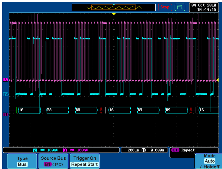
Fig. 7 Illustration of the GDS-3000 I 2 C decoding
