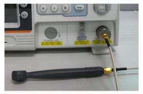
The GSP-9300 has various EMI test functions available, including the ability to test in high noise areas by pressing the Amb Noise soft-key, the ability to enter the antenna factor settings according to the type of antenna by pressing the Correction soft-key as well as applying limit line specifications by pressing the Recall Limit soft-key.
