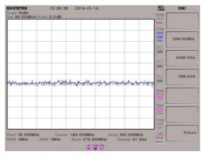
The GSP-9300 spectrum analyzer has a near field to far field conversion function that can be used when used in conjunction with these EMI probes. When the Correction soft-key is selected, noise in the near field can be converted to radiated field strength in the far field accordingly. This can this be used to determine whether the test product will be able to comply with the 3M far field test.
