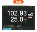
GOM-804/805 has two measurement speed selections, which are Fast reaching 60 readings per second, and Slow 10 readings per second. A major departure from the past, users, in the past, had to juggle between speed and display resolution. GOM-804/805 will not affect resolution despite of any speed selections and will maintain the highest display digits. In other words, reading resolution will not be changed by changing speed and the display digits remain the same.
