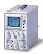
The GOS-310 10MHz Analog oscilloscope is design for Education, Student, Hobbyist and Maintenance use. Stadard Trigger Modes of Auto, Norm, Ext and TV sync. are provided and applicable in various market fields. High sensitivity of 5mV/div extends the measurement range and increases the test accuracy. The 10MHz bandwidth, single channel, 4.6kg light weight and compact size design make GOS-310 the best choice for affordable yet high performance oscilloscope.
