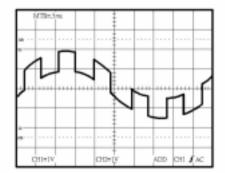
Figure 5-6 Typical ADD waveform
