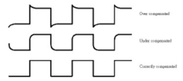
**Figure 5-2 Typical Compensation Waveform**
