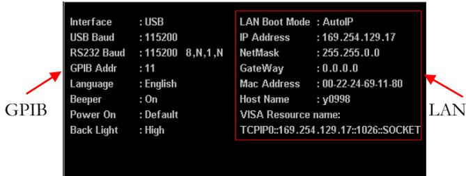
**Check operation** Press the System button on the panel to show the screen as above.
