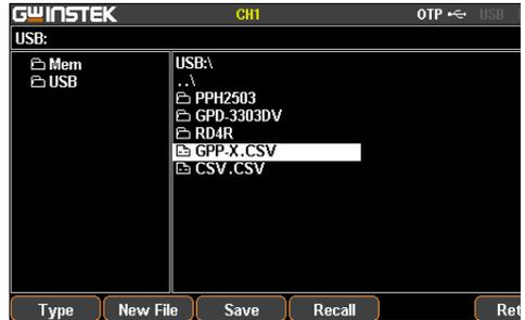
5. Press F3 (Save) button to save the settings of Sequence into the corresponding file.
