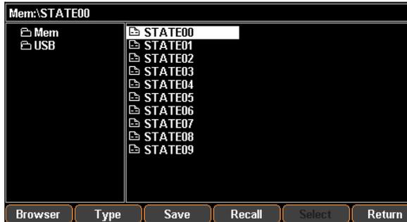
3. Press the F3 (Save) button to have the settings of current model saved into the corresponding file.
