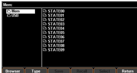
2. Press the right arrow button to enter the file group. Rotate the scroll wheel (Encode) and stop at the file in need
