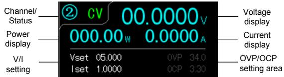
Channel no. Color of channel remains the original ① when not in the state of setting.
