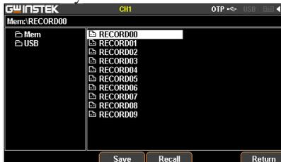
2. Press F3 (Save) button to save the temporary data into the corresponding file.
