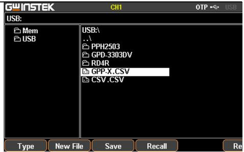
5. Press F3 (Save) button to save the settings of Delay into the corresponding file.
