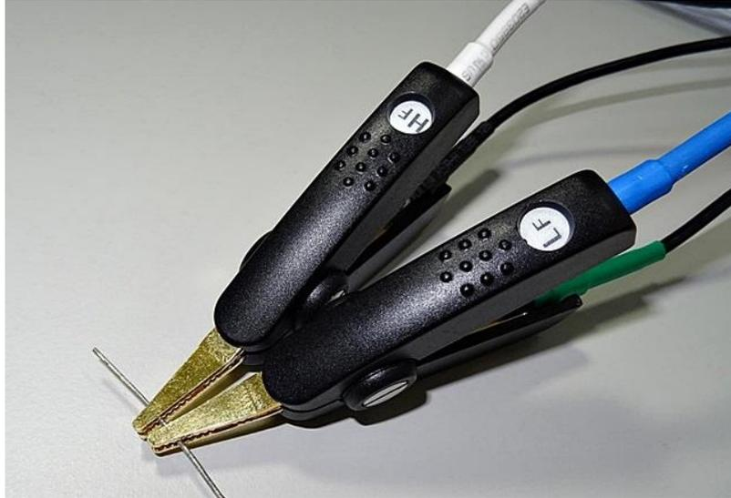
8. Press the [MEAS SHORT] soft-key and then the [OK] soft-key. Wait until the “Correction finished” message is displayed.
