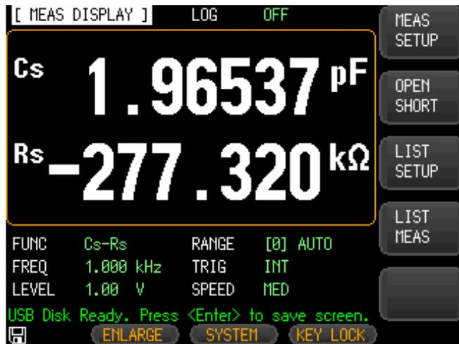
If the keypad is not needed to enter a numeric value, a screenshot of the meter's LCD display can be captured and saved to the USB disk by depressing the Enter key. If the screen shot is saved successfully, "Screen saved." will be shown in the message area at the bottom of the screen. The location and name of the screenshot will also be shown, for example: F:\LCR-6300\Screen\ScreenShot001.bmp.
