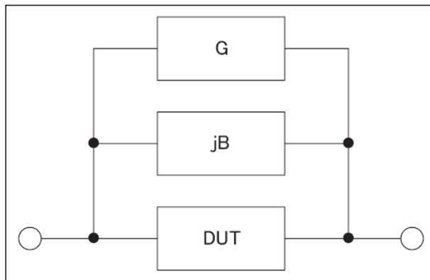
The OPEN correction data is taken at all preset frequency points, independent of the test frequency you set. Refer to the tables on page 128 for the trimming frequency point lists for each model.
