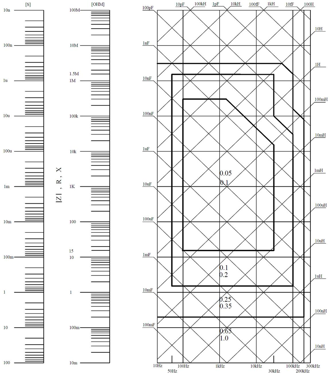
If the accuracy for the spot you are searching for falls right on the line, e.g. the horizontal thick line between values 0.25 and 0.65, then use the smaller value, 0.25, for the basic accuracy of the spot you are searching for.
