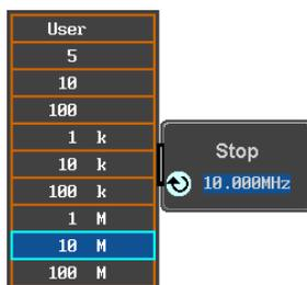
8. Alternatively, select *User* from the list of frequency or press the *Select* key. Use the arrows to select a base unit and the variable knob to further tune the selected base unit.
