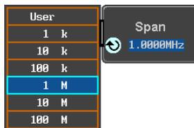
The variable knob can be used to select one. Press again on the *Span* button; the variable knob can now be used to set the frequency in increments of the chosen step resolution.
