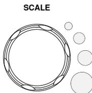
Sets the vertical scale of the channel (TIME/DIV).
