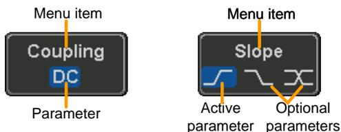
**Selecting a Menu Item, Parameter or Variable** When the user manual says to “select” a value from one of the side menu parameters, first press the corresponding menu key and use the Variable knob to either scroll through a parameter list or to increase or decrease a variable.
