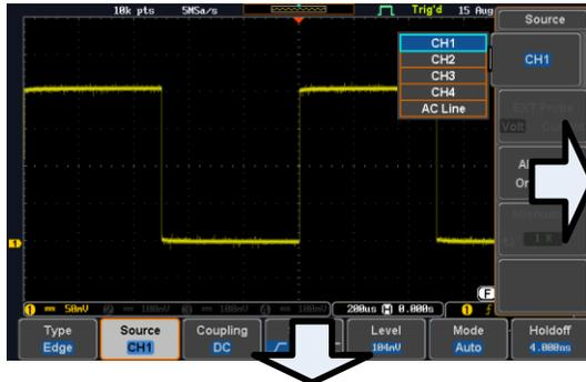
12. Press the *Menu Off* key to reduce the side menu, press again to reduce the bottom menu.
