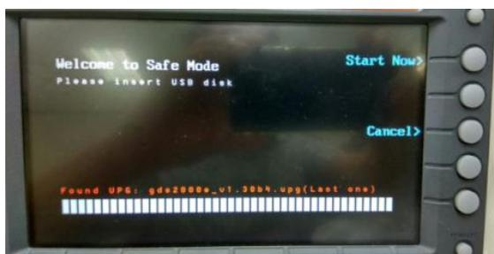
3. When the firmware file of USB flash disk has been recognized by oscilloscope, a message of "Found UPG: xxx.upg" will appear on the lower corner.
