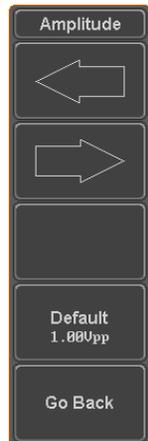
5. Default can be pressed to set the amplitude to 1.00Vpp.
