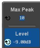
Select *Level* to set the threshold level for the search events. Any peaks above the threshold level will be seen as a search event.
