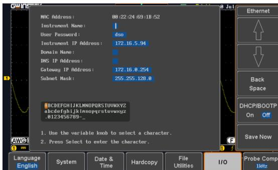
6. Use the *Up* and *Down* arrows on the side menu to navigate to each Ethernet configuration item.
