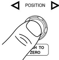
Alternatively, pressing the *Acquire* key and then pressing *Reset H Position to 0s* from the bottom menu will also reset the horizontal position.
