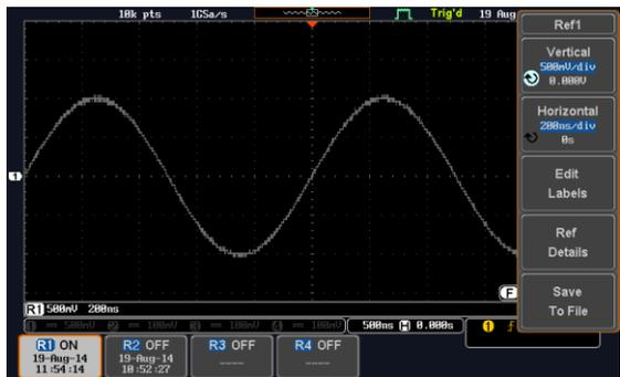
**Vertical Navigation**      Press *Vertical* repeatedly from the side menu to choose to edit the vertical position or Unit/Div. Use the Variable knob to edit the values.
