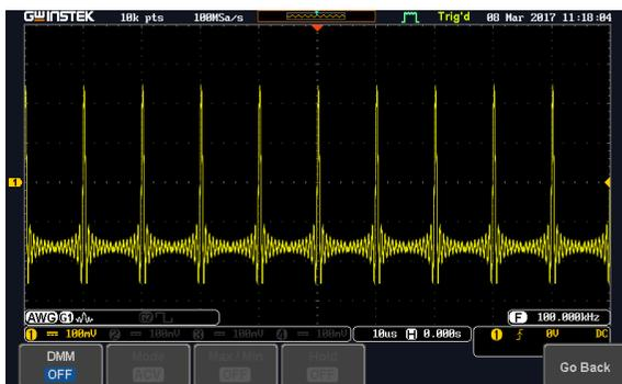
3. Press *DMM* button from the bottom menu to turn on the DMM function. You can select ACV, DCV, ACmV, DCmV, ACmA, DCmA, ACA, DCA, Ohms, Diode, Continuity and Temperature measurement from the DMM menu.
