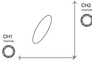
The horizontal position knob and horizontal Scale knob can still be used under the XY mode.
