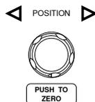
As the waveform moves, a position indicator on the top of the display indicates the horizontal position of the waveform in memory.
