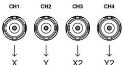
2. Make sure a channel pair is active (CH1&CH2 or CH3&CH4). Press the Channel key if necessary. A channel is active if the channel key is lit.
