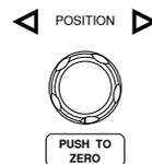
To reset the zoom position, press the *Horizontal Position* knob.
