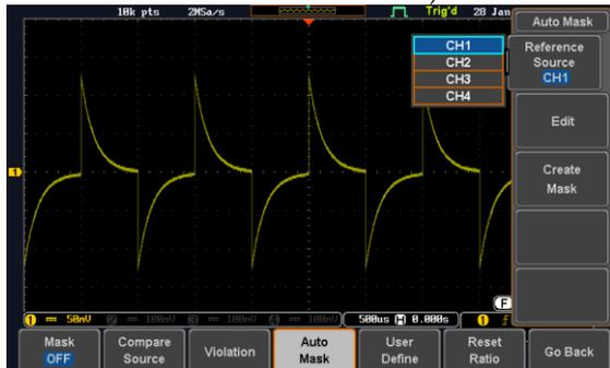
4. Press the *Edit* button from the side menu if you want to further adjust the mask pattern. Otherwise, go to step 9 below to create the mask directly without adjustment.
