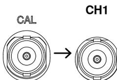
8. Press *Vertical* again after connecting CAL to the channel 1 input.
