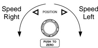
**Reset the Zoom Position** To reset both the zoom position and horizontal position, press *Reset Zoom & H POS to 0s*.
