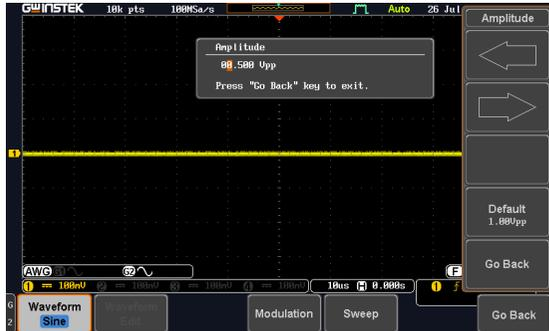
4. Use the Left and Right arrow keys to select a base unit and use the variable knob to increase the amplitude by that base unit, as shown in the Amplitude window.
