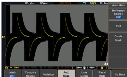
10. Press the *Auto Mask* button from the bottom menu to close auto mask function.
