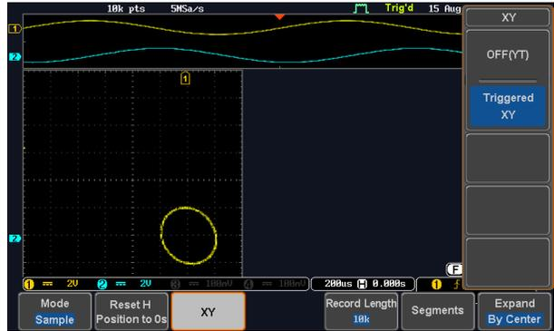
To move the XY waveform position, use the vertical position knob: Channel 1 knob moves the XY waveform horizontally and Channel 2 knob moves the XY waveform vertically. Similarly, the X2 and Y2 axis can be positioned using the channel 3 and channel 4 vertical position knobs.
