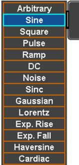
Selectable waveforms      Arbitrary, sine, square, pulse, ramp, DC, Noise, Sinc, Gaussian, Lorentz, Exp. Rise, Exp. Fall, Haversine, Cardiac.
