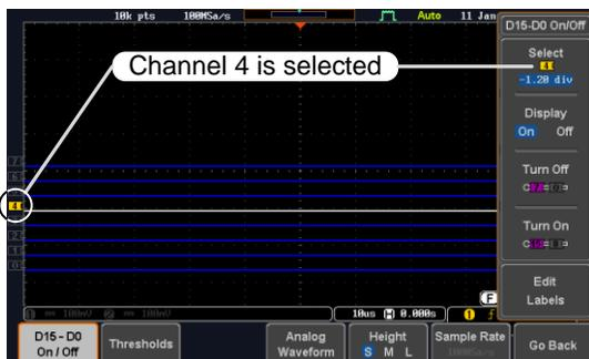
Note: If the Variable knob cannot select a channel, press the Select key to toggle the scope into 'LA Select mode'.
