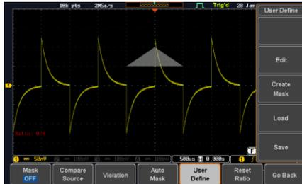
Note: Mask area must be defined clockwise sequentially. (Examples: two diagrams on the right)
