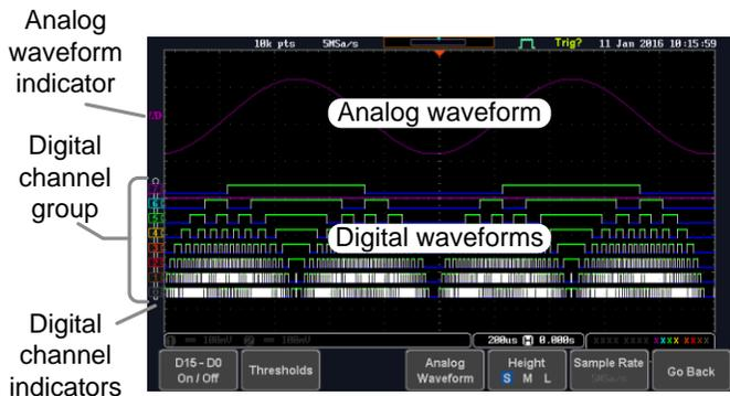
**Analog Waveform Indicator** Used to show the position of the analog waveform outputs.
