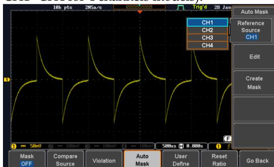
4. Press the *Edit* button from the side menu if you want to further adjust the mask pattern. Otherwise, go to step 9 below to create the mask directly without adjustment.
