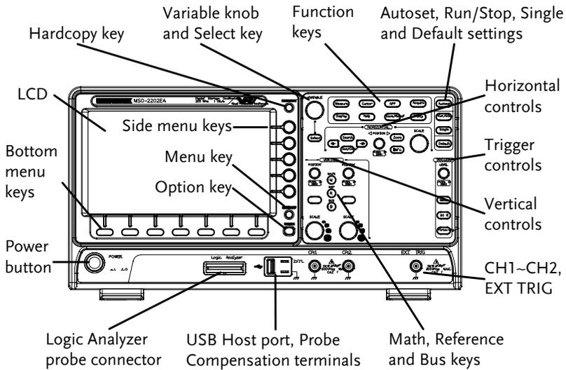
**LCD Display**      8" WVGA TFT color LCD. 800 x 480 resolution, wide angle view display.
