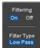
3. Press *Filter Type* and select low or high pass filter.
