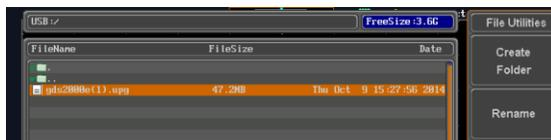
5. Press the *Select* key to begin the installation of the upgrade file.
