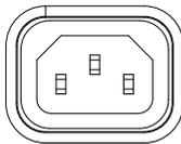
Power cord socket accepts AC mains, 100 ~ 240V, 50/60Hz.
