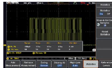
provides 8 measurement selections. The statistics mode can also be selected for users to analyze the mean value, the maximum, the minimum, and standard deviation of the retrieved waveforms to ensure signal's integrity and identify abnormal waveforms.
