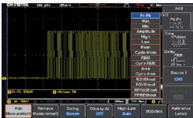
The MSO-2000E series soundly provides 38 measurement items. Based upon the parameters such as voltage, current, time, frequency, and delay measurement, users can decide which measurement items to choose. On the single display screen, the MSO-2000E series
