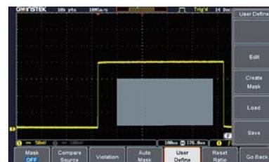
10 points to meet test requirements. Users can also refer to the examples from user manual to edit Mask by the PC to satisfy all test needs. By setting Save On, users can log and monitor signals, which violate test conditions.
