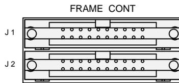
J1: The J1 connector is assigned to external control.
