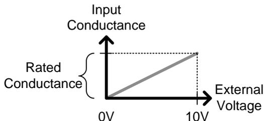
CV Mode                      Input voltage = rated voltage × (external
