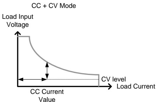
Note that when the source voltage is less than the CV level, no current will flow due to a very high impedance.
