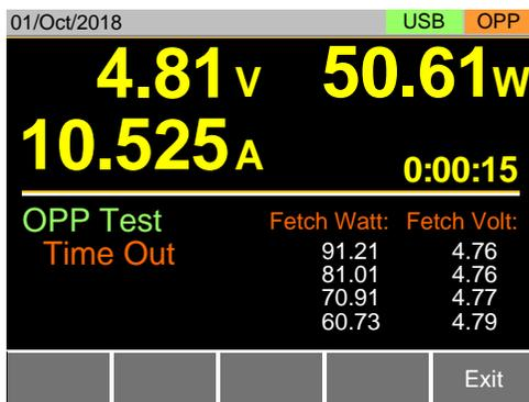
OPP time out will occur if the power supply's OPP fails to trigger. This is determined when the measured voltage is less than Trig V and the measured watt is greater than End W.
