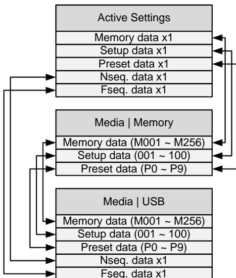
**Example** To load Preset Data P7 from USB, you must first load Preset Data P0-P9 to internal memory, then from internal memory load Preset P7 to be the
