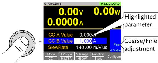
Cursor Mode: This method must first be enabled before it can be used. Pressing the scroll wheel when a parameter is highlighted allows you to set the step resolution by a digit value. An orange line will appear under the currently selected digit value. Repeatedly pressing the scroll wheel moves to the next digit. See page 79 for details.
