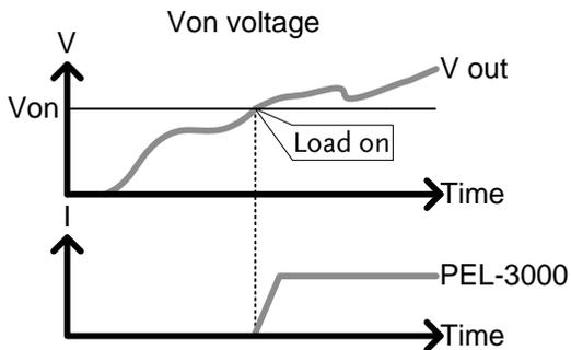
**Operation** 2. Press **Main** > *Configure*[F5] > *Other*[F2] and set the *Von Voltage* level.
