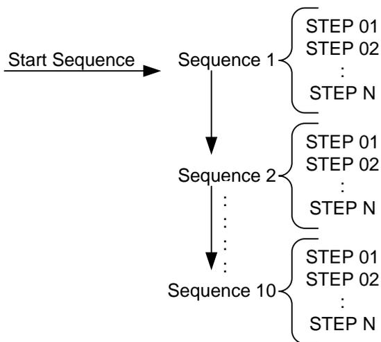
**Description** Normal Sequence configuration is split into Timing Edit configuration and Data Edit configuration.
