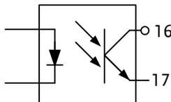
Photocoupler input: 30V max, 8mA, max.
