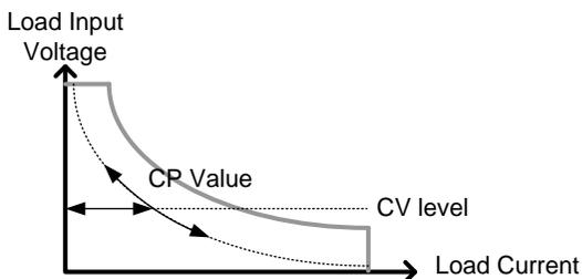
Note that when the source voltage is less than the CV level, no current will flow due to a very high impedance.
