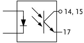
Photocoupler input: 30V max, 8mA, max.
