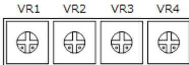
The variable resistors are used to adjust the full scale and offset setting for the input value of the external control sources such as voltage or resistance.
