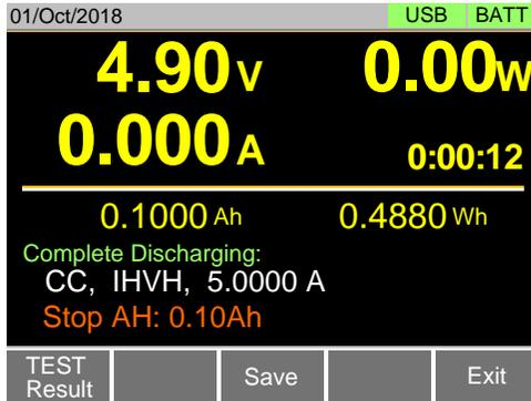
The BATT Test will return the information of the last discharge when the Battery stop voltage or stop time or stop AH was tripped.
