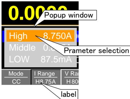
Parameter Input      The scroll wheel, Enter key and number pad can be used to edit parameter values.
