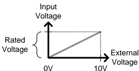
CP Mode                      Input power = rated power × (external voltage/10)
