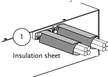
2. Secure the insulation sheets using the supplied velcro fasteners. 2 fasteners should be used for each sheet.
