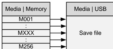
For example, Memory Data M001 to M256 are saved to a single file on USB.
