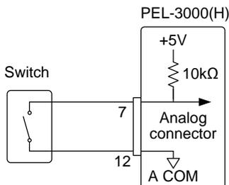
**Example** The LoadOn IN setting determines whether the load is turned on when the external switch is closed (low) or open (high).
