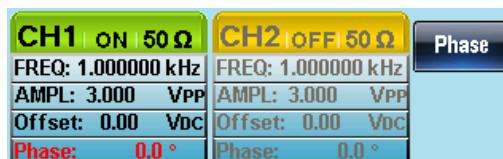
4. Use the arrow keys and scroll wheel or number pad to enter the output phase.
