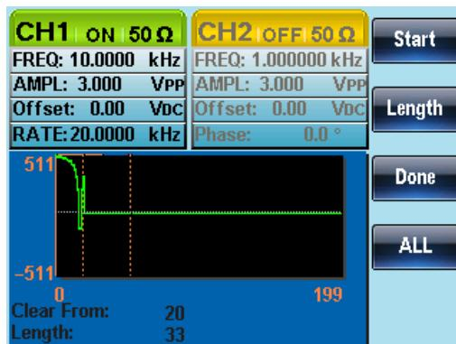
The result after the whole waveform is deleted:
