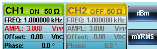
3. Use the arrow keys and scroll wheel or number pad to enter the amplitude.
