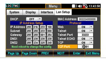
18. Use the Left/Right keys to move the cursor followed by scrolling Knob key or pressing +/- keys to define TCP Port. Also, you can press Number keys to directly input a specific digit.
