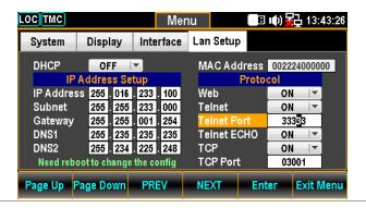
Use the Left/Right keys to move the cursor followed by scrolling Knob key or pressing +/- keys to define Telnet Port. Also, you can press Number keys to directly input a specific digit.
