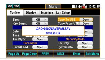
5. The prompt message pops up and indicates the file of parameters is saved to the connected USB completely.
