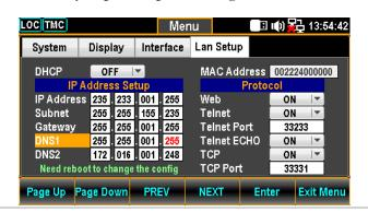
16. Press the F5 (Enter) key or Knob key again to confirm the input digit for D11. And the cursor will automatically jump to next groups.
