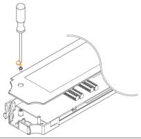
2. With help of a Phillips-head screwdriver, connect the wire to the terminal followed by routing the wire to the end port of module.
