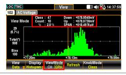
4. Due to readings are not updated with the live scan in histogram display, press the *Refresh* (F4) key to update live readings when a scan course is ongoing.
