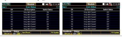
4. When user intends to carry out firmware update for installed module, press the *FW Update* (F6) key to perform update process. The prompt message pops up and user can press *Yes* (F1) to carry on the update.
