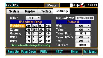
3. Use the Left/Right keys to move the cursor followed by scrolling Knob key or pressing +/- keys to define IP Address. Also, you can press Number keys to directly input a specific digit.
