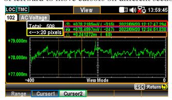
White Sect. The total counts of scanned measurements.
