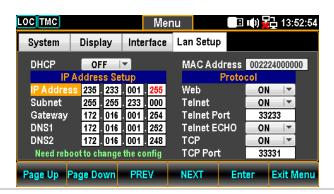
4. Press the F5 (Enter) key or Knob key to confirm the input digit for IP1 Address. And the cursor will automatically jump to next groups.
