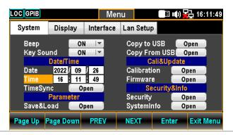
2. Use the Left/Right keys to move the cursor followed by scrolling Knob key or pressing +/- keys to define hour of Time. Also, you can press Number keys to directly input a specific digit.
