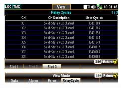
2. Use the *knob* key to navigate through pages to have view on the number of cycles of each relay from different channels.
