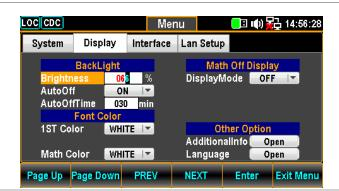
3. Press the F5 (Enter) key or Knob key to confirm the input digit for backlight brightness.
