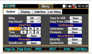
2. Use the Left/Right keys to move the cursor followed by scrolling Knob key or pressing +/- keys to define year of Date. Also, you can press Number keys to directly input a specific digit.
