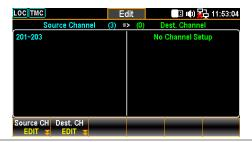
4. Use *knob* key to navigate channels followed by pressing *Select* or *Select All* to select destination channels. Press *Cancel* or *Clear All* to deselect channels. Press *OK* to confirm selection. Press *Exit* to leave the page without saving the selection.
