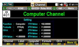
2. Press the (x)TH (F1) key to select a coefficient order (0TH, 1TH, 2TH, 3TH, 4TH, 5TH) followed by pressing the TH Value (F2) key to configure parameters for each coefficient order.
