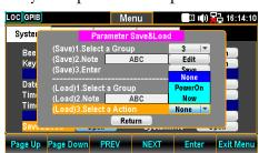
5. Scroll the Knob key or press +/- keys followed by pressing the F5 (Enter) key or Knob key to confirm the action selection.
