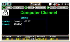
2. Use *knob* key to navigate channels. Press the *Select* (F5) key to select a channel followed by press the OK (F4) key to confirm all selections. If a channel is selected, press the *Cancel* (F5) key to deselect a channel or press the *ClearAll* (F3) key to deselect all channels. Press the *Exit* (F6) key to leave without saving.
