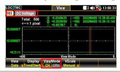
3. When the "GRH" is selected for *ViewMode* (F3) key, scroll the *knob* key to navigate through scanned counts. If pressing *knob* key, the maximum counts moving by scrolling *knob* key per time will be changed.
