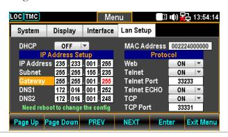
12. Press the F5 (Enter) key or Knob key to confirm the input digit for G1. And the cursor will automatically jump to next groups.
