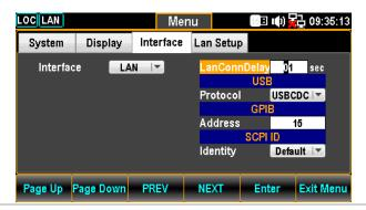
3. Use the Left/Right keys to move the cursor followed by scrolling Knob key or pressing +/- keys to set LAN Connect Delay Time. Also, you can press Number keys to directly input a specific digit.
