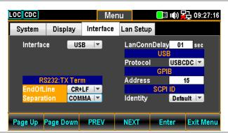
11. Press the F5 (Enter) key or Knob key followed by scrolling Knob key or pressing +/- keys to land on the desired option of Separation field.
