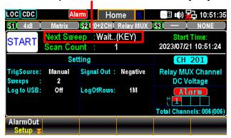
External It indicates a trigger signal received from the rear panel to start each sweep for a scan course. Press the *TrigSignal* (F2) key to configure the polarity of external signal in either Pos or Neg.
