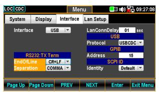
8. Press the F5 (Enter) key or Knob key followed by scrolling Knob key or pressing +/- keys to land on the desired option of EndOfLine field.
