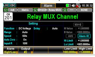
2. Press the *Alarm* (F1) key to select an alarm limit(s) mode to report for select channel.
