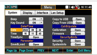
3. Press the F5 (Enter) key or Knob key to confirm the input digit for year of Date.
