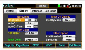
2. Use the Left/Right keys to move the cursor followed by scrolling Knob key or pressing +/- keys to define digit. Also, you can press Number keys to directly input a specific digit.
