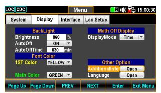
3. Press the F5 (Enter) key or Knob key to enter the Additional menu. Press the Next key or scroll the Knob key followed by pushing the F5 (Enter) key or Knob key to enable/disable each option. Move to the Return option followed by pressing the F5 (Enter) key or Knob key to have the setting take effect.
