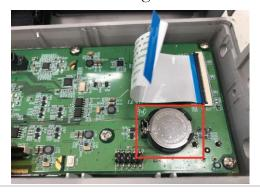
4. Gently remove the battery via the end tip of flat-head screwdriver as the following figure shown.
