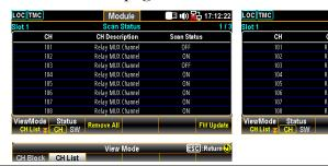
3. If any channel is set Switch mode, press the *Status* (F2) key to select SW followed by pressing the *Card Reset* (F3) key to reset the select module. All channels on the module will be opened. Refer to page 85 for details of Switch mode.
