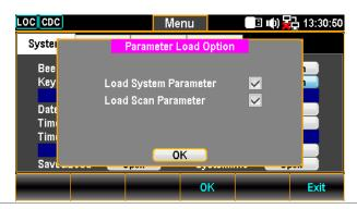
5. Scroll the Knob key to move between System and Scan Parameters followed by pressing Knob key to select/unselect parameters. Press F4 (OK) key to load parameters to DAQ-9600.
