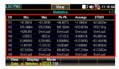
4. Press the *Mode* (F3) key to toggle between STAT (Statistics) and TIM (Time Stamp) displays. The TIM mode displays the Date & Time of Minimum and Maximum readings of each channel from a scan course.
