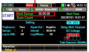
Manual It indicates a manual trigger. When selecting this method, user needs to press the *Scan* key on the front panel to start each sweep for a scan course.
