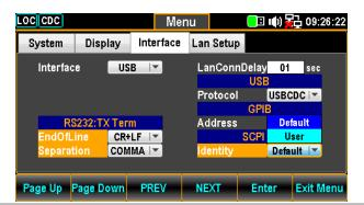
4. Press the F5 (Enter) key or Knob key again to confirm the desired SCPI ID Identity option
