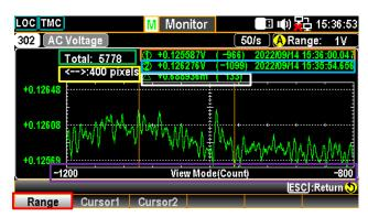
Green The total counts of measurements Sect. before entering the Stop&View.
