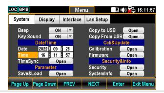
3. Press the F5 (Enter) key or Knob key to confirm the input digit for hour of Time.
