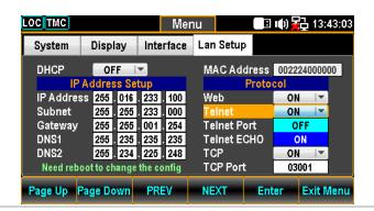
7. Press the F5 (Enter) key or Knob key to confirm the Telnet ON option.
