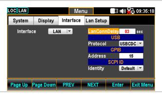
4. Press the F5 (Enter) key or Knob key again to confirm the LAN Connect Delay Time.
