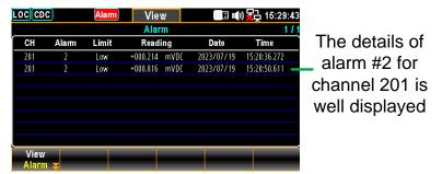
Alarm in Under the Monitor mode, if set limit of alarm is exceeded, the Monitor mode color of reading becomes warning red in different display modes.
