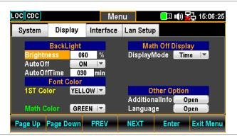
2. Press the NEXT key repeatedly or scroll the Knob key to move to the BackLight – AutoOffTime field.
