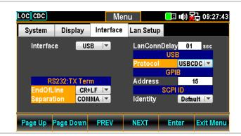
5. Press the F5 (Enter) key or Knob key followed by scrolling Knob key or pressing +/- keys to land on the desired USB Protocol option.
