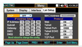
2. Press the F4 (NEXT) key repeatedly or scroll the Knob key to move to the IP Address Setup – IP Address field.
