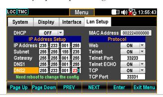
20. Press the F5 (Enter) key or Knob key again to confirm the input digit for D21. And the cursor will automatically jump to next groups.
