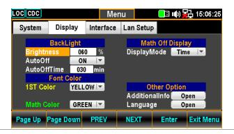
2. Press the NEXT key repeatedly or scroll the Knob key to move to the BackLight - AutoOff field.
