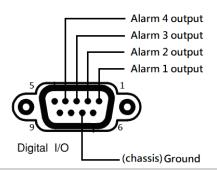
Pin1-4 Alarm output pins
