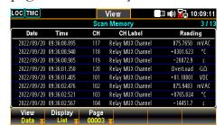
3. The list mode displays Date, Time, Channel, Channel Label (naming by user) and reading of each measured data from a scan course.
