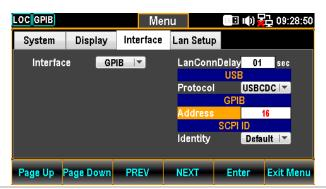
6. Press the F5 (Enter) key or Knob key again to confirm the input digit for GPIB Address.
