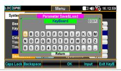
5. Use the Left/Right and +/- keys or scroll the Knob key to move the cursor to desired word followed by pressing the F5 (Input) key or Knob key to input the word.
