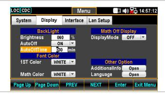
3. Use the Left/Right keys to move the cursor followed by scrolling Knob key or pressing +/- keys to define minutes. Also, you can press Number keys to directly input a specific minutes.
