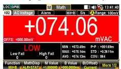
Values Left Sec. The numbers of High and Low limits exceeding are shown individually. Right Sec. The values, which based on MX+B calculation, identical to STAT page are well displayed.
