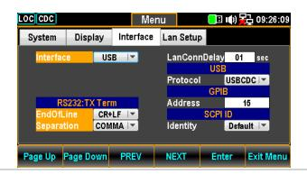
2. Press the F5 (Enter) key or Knob key followed by scrolling Knob key or pressing +/- keys to land on the GPIB option.
