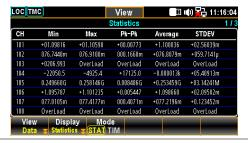
3. The statistics mode displays Channel, Minimum, Maximum, Pk-Pk (Peak-to-Peak), Average and STDEV (Standard Deviation) of readings data from a scan course.
