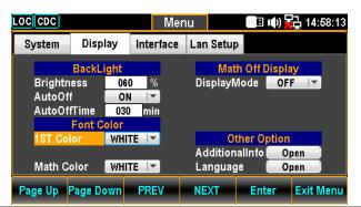
3. Press the F5 (Enter) key or Knob key followed by scrolling Knob key or pressing +/- keys to select desired color for 1ST display.
