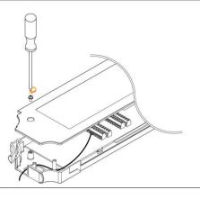
4. Insert the module into one of the module slots from the rear panel of DAQ-9600 unit.
