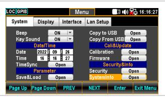
2. Press the F5 (Enter) key or Knob key to enter the System Information where all the critical contents are exposed for check.
