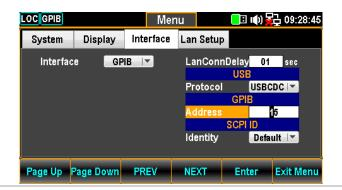
5. Use the Left/Right keys to move the cursor followed by scrolling Knob key or pressing +/- keys to define GPIB Address. Also, you can press Number keys to directly input a specific digit.
