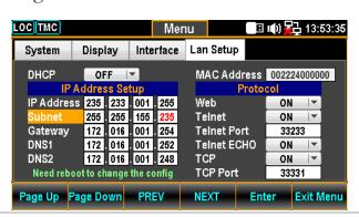
8. Press the F5 (Enter) key or Knob key again to confirm the input digit for S1. And the cursor will automatically jump to next groups.
