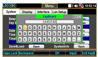
Use the Left/Right and +/- keys or scroll the Knob key to move the cursor followed by pressing the F5 (Input) key or the Knob key to specify a name for parameters.
