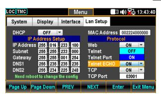
13. Press the F5 (Enter) key or Knob key again to confirm the Telnet ECHO ON option.
