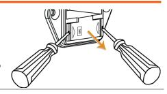
2. The fuse socket appears. The "240" symbol within the hole on fuse socket indicates the line voltage is positioned as 240V.
