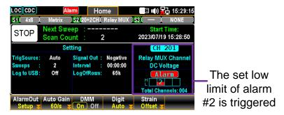
6. Also, the alarm details will be saved in the memory when the set alarm occurs for select channel during a scan course. Press the *View* key on the front panel to view the info of triggered alarm. Refer to page 100 for details of View menu.
