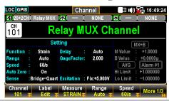
2. Press the *Module* key from the front panel followed by clicking the *ViewMode* key and then *CH List* key.
