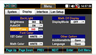
4. Press the F5 (Enter) key or Knob key to confirm the input minutes for Auto Off Time.
