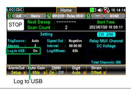
3. Press the # Rows (F3) key to specify the row limit, which indicates the max. number of rows for sweep data, of each data logging file. The "65k" means the limit is 65,536 rows per file. The "1M" indicates the limit is 1,048,576 rows per file and the "Infinite" stands for the limit varies based on the number of bytes permitted by file system itself.
