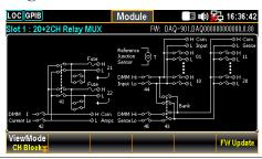
2. Press the *ViewMode* (F1) key followed by pressing the *CH List* (F2) key. And the Scan Status of all channels from select module will be shown. Scroll the *knob* key to navigate through pages of different channels. Press *Remove All* (F3) key to remove the set measurements of all channels at once. Refer to page 51 for details of Switch mode.
