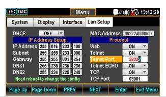
10. Press the F5 (Enter) key or Knob key to confirm the input digit for Telnet Port.
