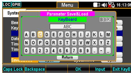
6. Press the F4 (OK) or the Knob key to confirm the input words.
