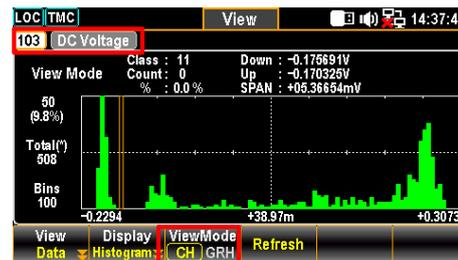
3. When the “GRH” is selected for *ViewMode* (F3) key, scroll the *knob* key to navigate through each scanned count.
