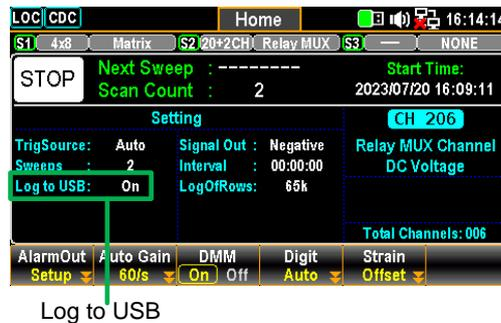
3. Press the *# Rows* (F3) key to specify the row limit, which indicates the max. number of rows for sweep data, of each data logging file. The “65k” means the limit is 65,536 rows per file. The “1M” indicates the limit is 1,048,576 rows per file and the “Infinite” stands for the limit varies based on the number of bytes permitted by file system itself.
