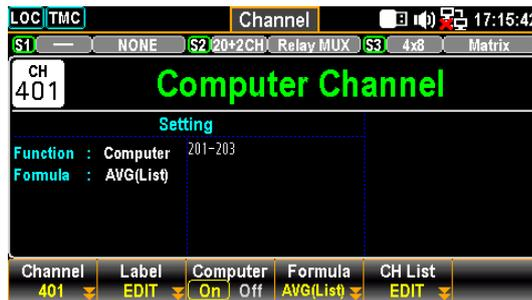
2. Use *knob* key to navigate channels. Press the *Select* (F5) key to select a channel followed by press the OK (F4) key to confirm all selections. If a channel is selected, press the *Cancel* (F5) key to deselect a channel or press the *ClearAll* (F3) key to deselect all channels. Press the *Exit* (F6) key to leave without saving.
