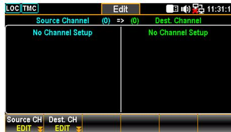
2. Use *knob key* to navigate channels followed by pressing *Select* or *Select.All* to select source channels. Press *Cancel* or *Clear.All* to deselect channels. Press *OK* to confirm selection. Press *Exit* to leave the page without saving the selection.
