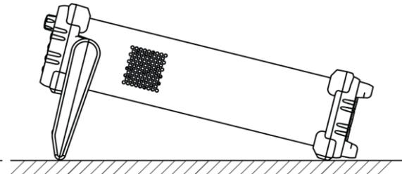
Rotate the handle for tilt stand.
