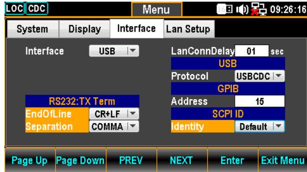
3. Press the F5 (Enter) key or Knob key followed by scrolling Knob key or pressing +/- keys to land on the desired SCPI ID Identity option.
