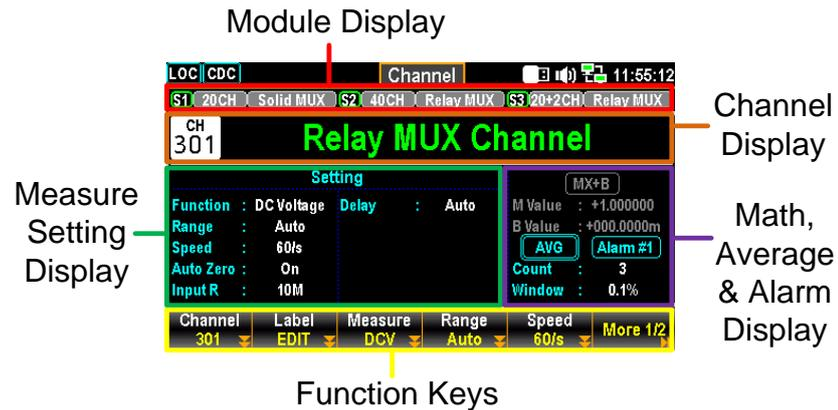
**Module Display** It includes module slot number and module name as well as total channels of each module. Up to 3 installed modules can be displayed.
