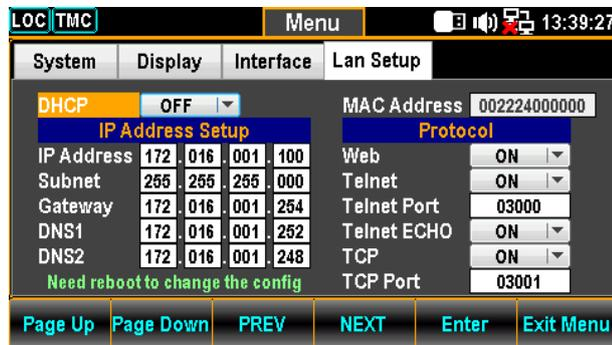
2. Press the F4 (NEXT) key repeatedly or scroll the Knob to move to the IP Address Setup – IP Address field.
