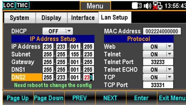
20. Press the F5 (Enter) key or Knob key again to confirm the input digit for D21. And the cursor will automatically jump to next groups.
