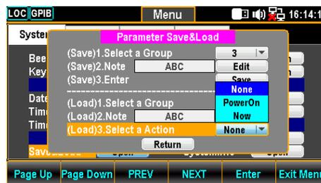
5. Scroll the Knob key or press +/- keys followed by pressing the F5 (Enter) key or Knob key to confirm the action selection.
