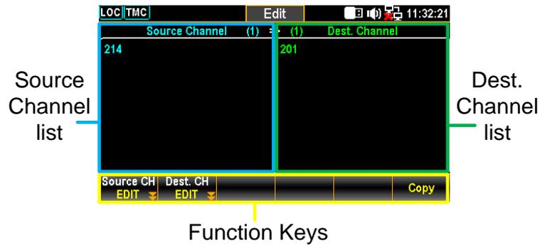
**Source Channel** The channels selected as source are displayed in detail within the lower list section and the upper section indicates the total number of source channels selected.
