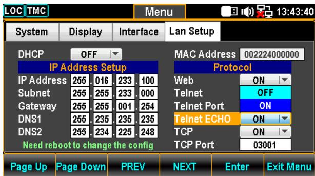
13. Press the F5 (Enter) key or Knob key again to confirm the Telnet ECHO ON option.
