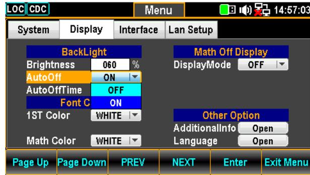
4. Press the F5 (Enter) key or Knob key to confirm the ON option for AutoOff.
