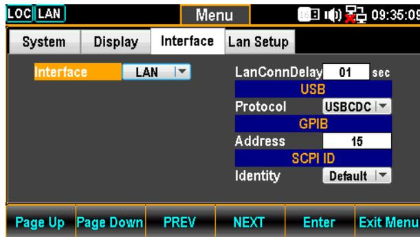
2. Press the F4 (NEXT) key repeatedly or scroll the Knob key to move to LAN Connect Delay Time.
