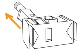
4. Further pull the fuse out of the fuse holder and replace it with a new fuse.
