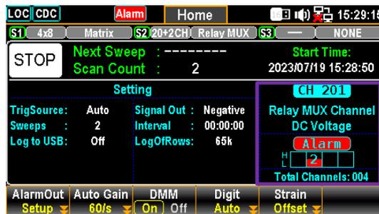
The set low limit of alarm #2 is triggered
