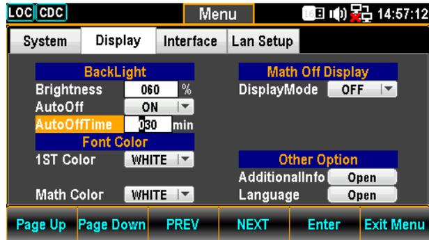
3. Use the Left/Right keys to move the cursor followed by scrolling Knob key or pressing +/- keys to define minutes. Also, you can press Number keys to directly input a specific minutes.
