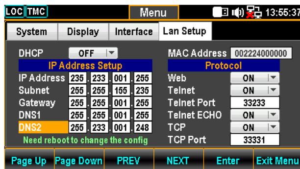
19. Use the Left/Right keys to move the cursor followed by scrolling Knob key or pressing +/- keys to define DNS2. Also, you can press Number keys to directly input a specific digit.
