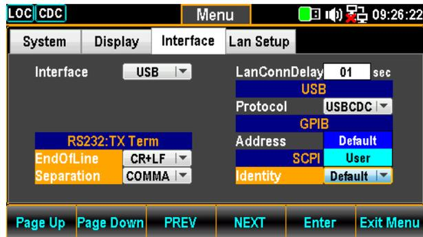
4. Press the F5 (Enter) key or Knob key again to confirm the desired SCPI ID Identity option
