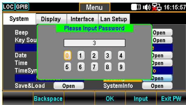
3. Use the Left/Right and +/- keys or scroll the Knob key to move the cursor followed by pressing the F5 (Input) key or the Knob key to input the password.
