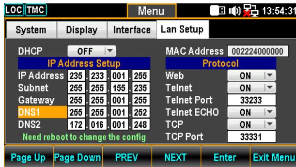
15. Use the Left/Right keys to move the cursor followed by scrolling Knob key or pressing +/- keys to define DNS1. Also, you can press Number keys to directly input a specific digit.
