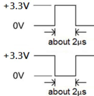
Pin6 External Trigger Input. Accepts external trigger signals. For using external signals.
