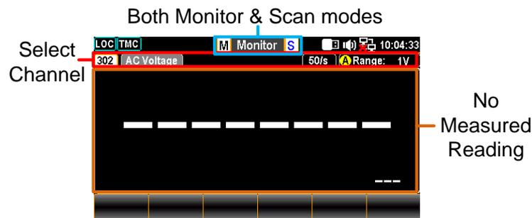
When the select channel is being scanned from a sweep within a scan course, measured reading will be displayed and be updated again only when being scanned again in the next sweep.
