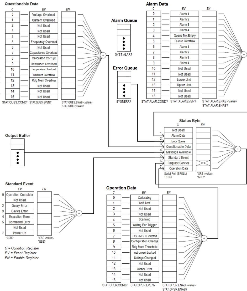
NOTE: The overload bits are set once per INITiate command. If you clear an overload bit, it is not set again until a new INITiate is sent.
