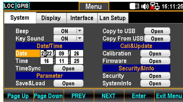
2. Use the Left/Right keys to move the cursor followed by scrolling Knob key or pressing +/- keys to define year of Date. Also, you can press Number keys to directly input a specific digit.
