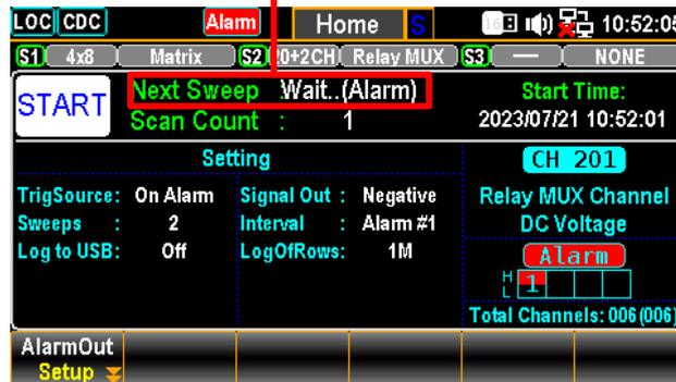
F2 (Time) key to set interval When Time of TrigSource is selected, press the key to specify a time interval.
