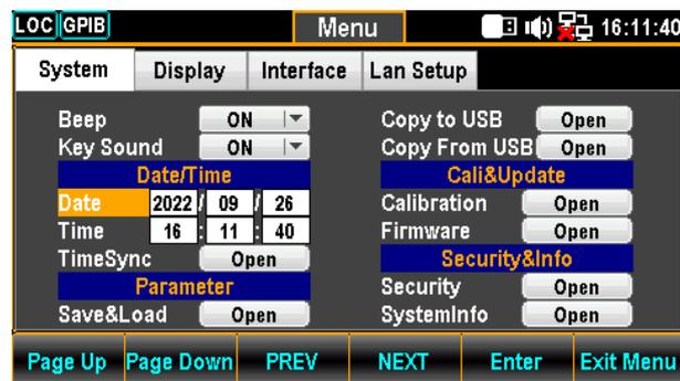
3. Press the F5 (Enter) key or Knob key to confirm the input digit for year of Date.
