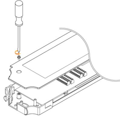
2. With help of a Phillips-head screwdriver, connect the wire to the terminal followed by routing the wire to the end port of module.
