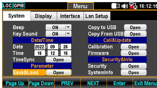
2. Press the F5 (Enter) key or Knob key to enter the Parameter Save&Load menu.
