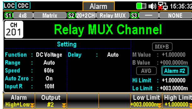
2. Press the *Alarm* (F1) key to select an alarm limit(s) mode to report for select channel.
