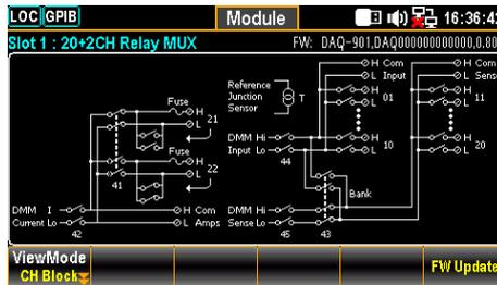
2. Press the *ViewMode* (F1) key followed by pressing the *CH List* (F2) key. And the Scan Status of all channels from select module will be shown. Scroll the *knob* key to navigate through pages of different channels. Press *Remove All* (F3) key to remove the set measurements of all channels at once. Refer to page 51 for details of Switch mode.
