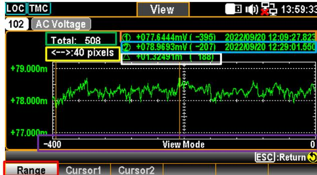
Green Sect. The total counts of scanned measurements.
