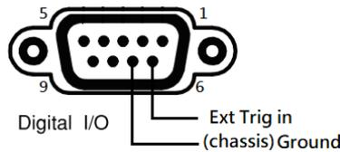
**Pin6** External Trigger Input pin
