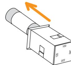
5. Restore the fuse holder with new fuse back to the fuse socket. Ensure that the correct line voltage shows within the hole of the fuse socket per requirement.
