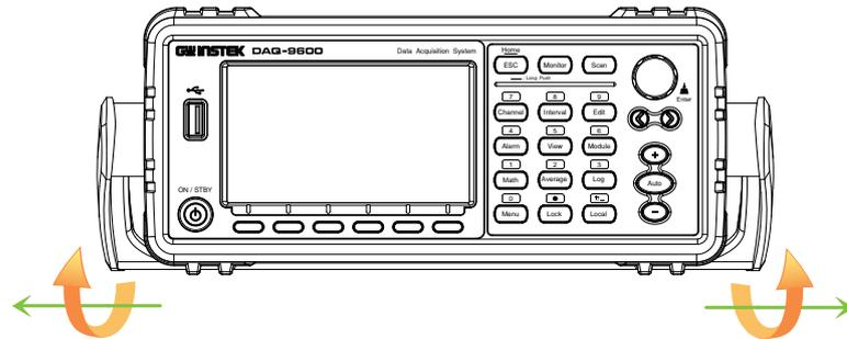
Pull out the handle sideways and rotate it clockwise for the applications below.
