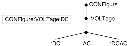
**Command Types** There are a number of different instrument commands and queries. A command sends instructions or data to the unit and a query receives data or status information from the unit.
