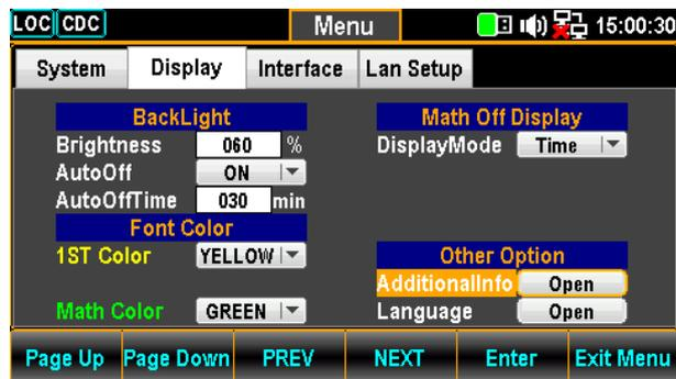
3. Press the F5 (Enter) key or Knob key to enter the Additional menu. Press the Next key or scroll the Knob key followed by pushing the F5 (Enter) key or Knob key to enable/disable each option. Move to the Return option followed by pressing the F5 (Enter) key or Knob key to have the setting take effect.
