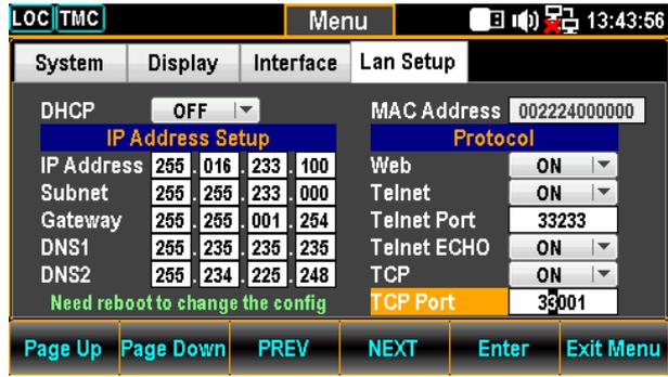
18. Use the Left/Right keys to move the cursor followed by scrolling Knob key or pressing +/- keys to define TCP Port. Also, you can press Number keys to directly input a specific digit.
