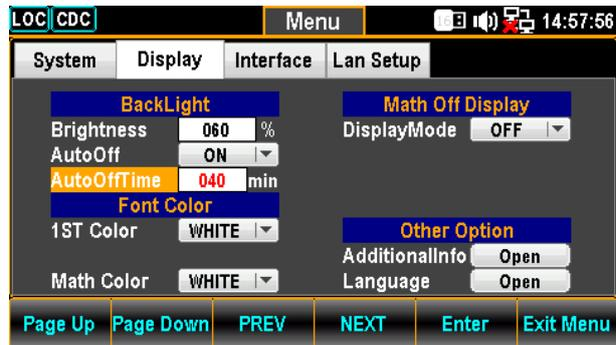
4. Press the F5 (Enter) key or Knob key to confirm the input minutes for Auto Off Time.
