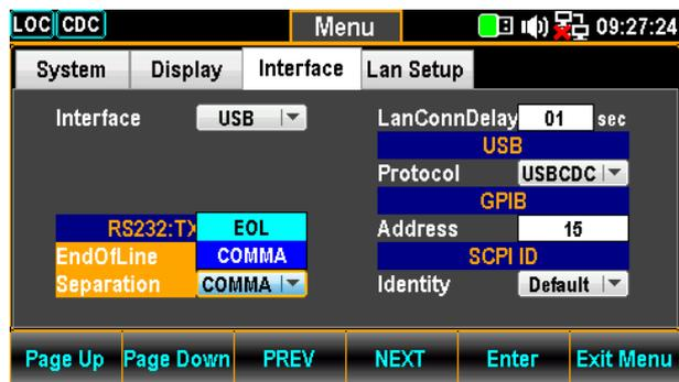
12. Press the F5 (Enter) key or Knob key again to confirm the selected option of Separation field.
