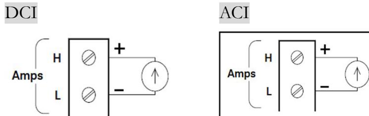
**F4 (Range) key to select range for ACI and DCI** Press the key to enter Range menu and select a target range for ACI and DCI measurements individually. The Auto indicates a range, which is based on the source input, is selected automatically. It is sometimes results in, compared with manual select range, slower measurement. Also, using the *Range* keys can select range promptly.
