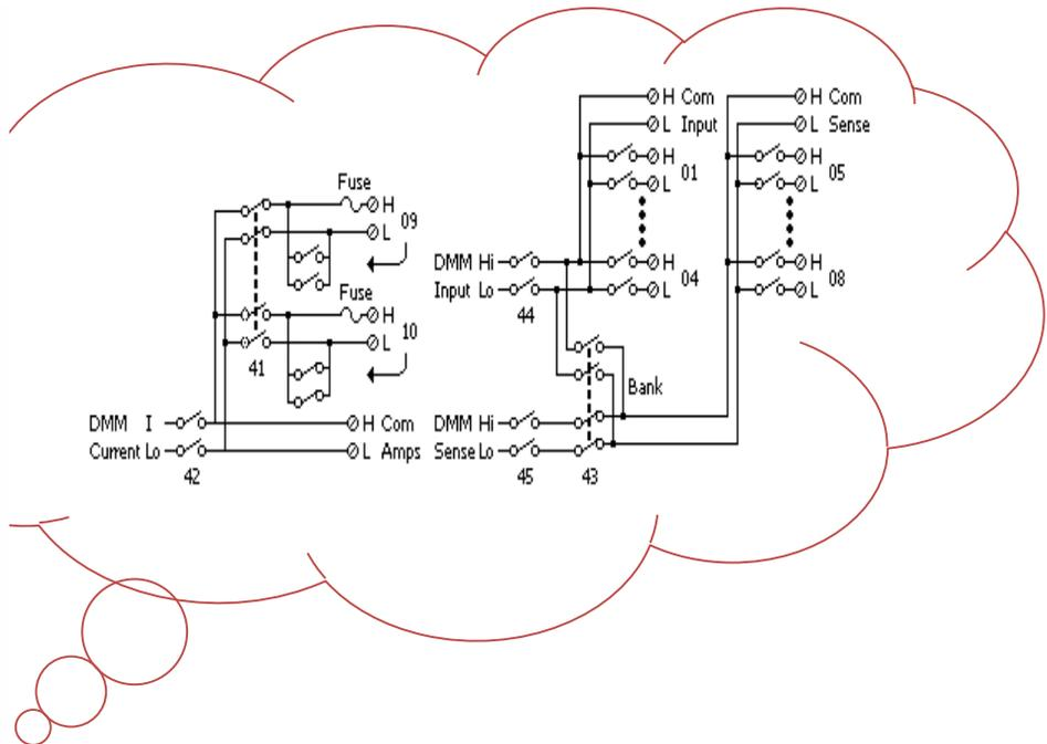
DAQ-909 is a multiplexer specially designed for high voltage, providing 8 channels for DC 600V / AC 400Vrms voltage measurement. The additional 2 current input channels can be used for AC and DC current measurement, external shunt resistors are not required (maximum 2A / per channel).
