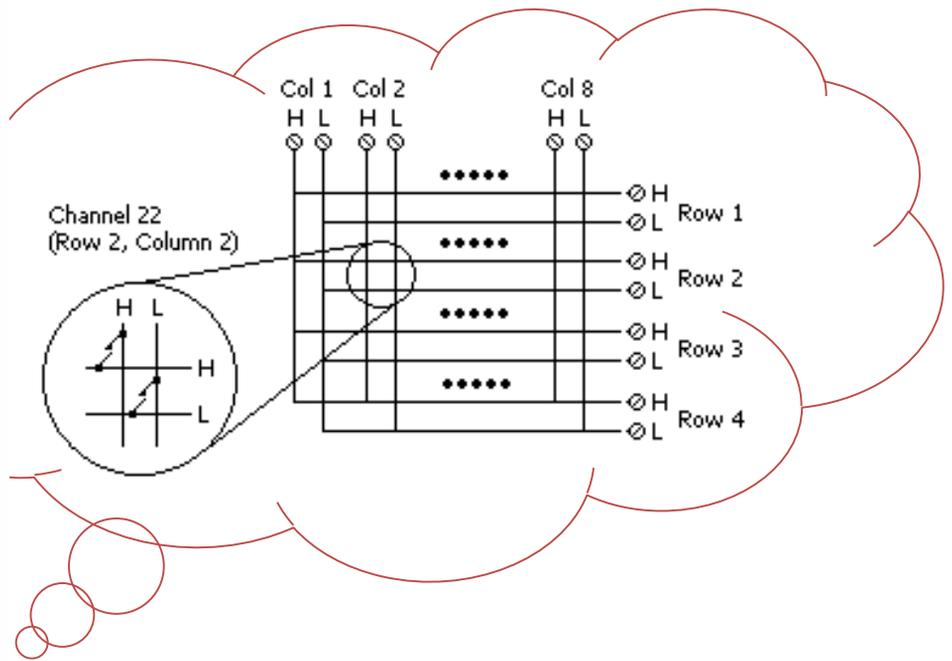
DAQ-904 module can provide the most flexible connection path between your DUT and the test system, allowing different test instruments to be connected to multiple points on the DUT at the same time.
