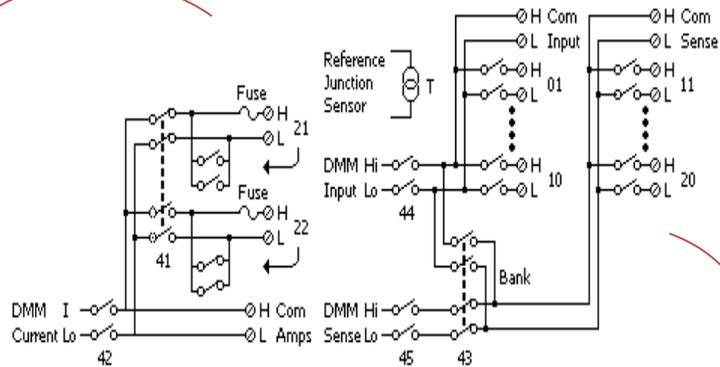
DAQ-901 is a comprehensive multiplexer for general scanning. The same module can mix 2-wire and 4-wire channels; at the same time, the additional 2 current input channels can be used for AC and DC current measurement without external shunt resistors (maximum 1A per channel).
