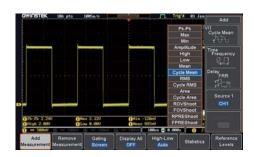
The GDS-1000B series oscilloscope is equipped with 36 different automatic measurement parameter functions. Users, after obtaining measured waveforms, can select different measurement parameters from Measure key according to different measurement requirements. The GDS-1000B Series shows simultaneously eight sets of different measurement parameters on the bottom of the
