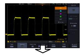
12. Press the relevant function key again to reduce the bottom menu. For example: press the Trigger Menu key to reduce the trigger menu.
