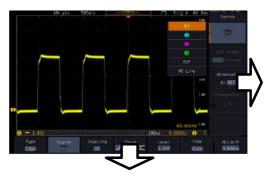
13. Press the *Menu Off* key to reduce the side menu, press again to reduce the bottom menu.
