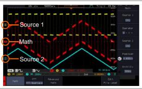
Position and Unit To move the math waveform vertically, press the *Position* key from the side menu and use the *VARIABLE* knob to set the position.
