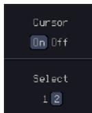
Move the active cursor along the active trace using the *VARIABLE* knob. The corresponding frequency value in Hz (X-axis), gain value in dB (left Y-axis) and phase value in degree (right Y-axis) messages are shown below.
