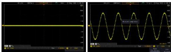
3. To undo Autoset, press *Undo Autoset* from the bottom menu.
