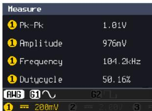
**Choose a Source** The channel source for measurement items can be set either before or when selecting a measurement item.
