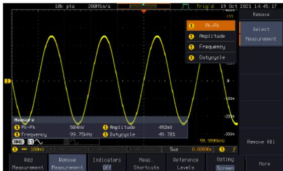
Remove All Items Press *Remove All* to remove all the measurement items.
