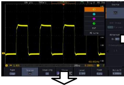
13. Press the *Menu Off* key to reduce the side menu, press again to reduce the bottom menu.
